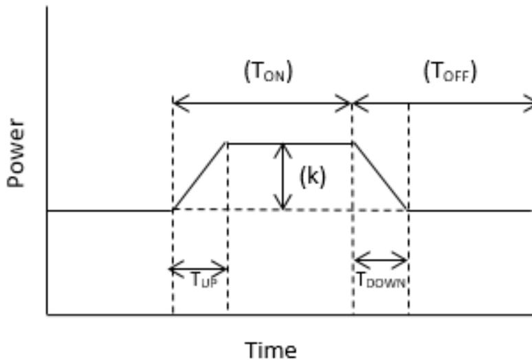
Figure 1: Extended Fluid Flow ON-OFF Model
