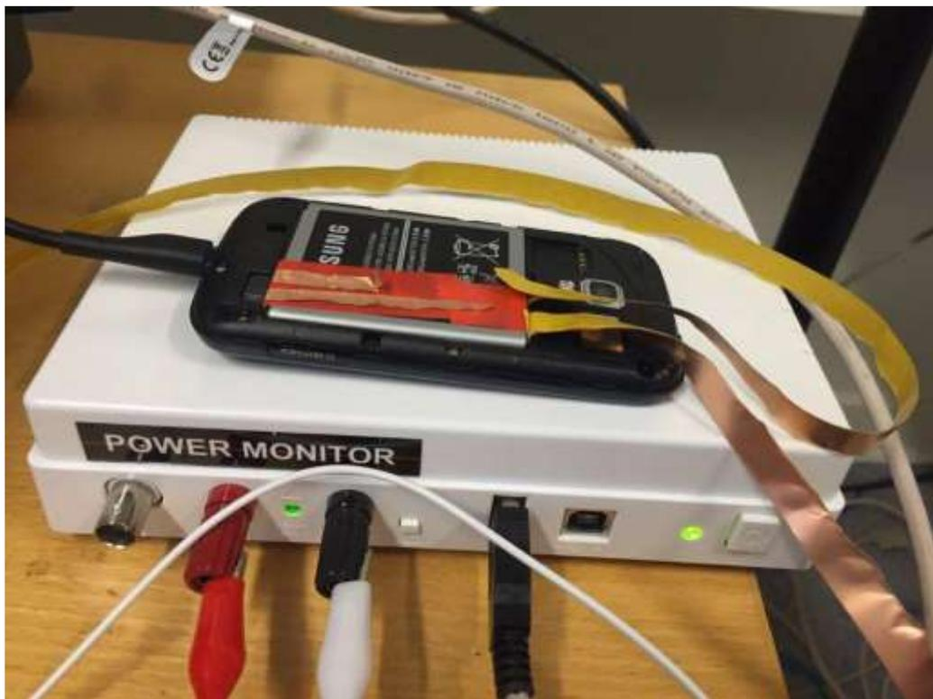
*Figure 6 Power Monitor Connections*
