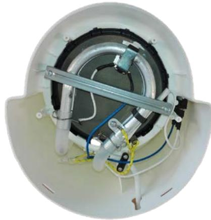
*Figure 2-2 Heating system*
