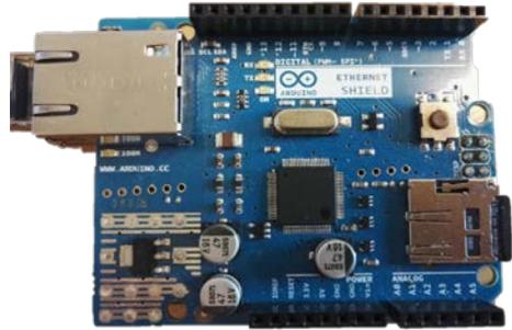
Figure 2-5 Ethernet shield
