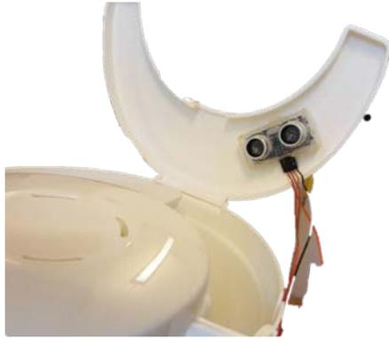
Figure 4-12 Position of Ultrasonic sensor
