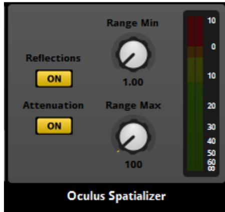
Figure 4. The Oculus plugin in the middleware FMOD studio. To the right is an output meter displaying the outgoing signal to the program's mixer, the two knobs represent minimum and maximum attenuation value.
