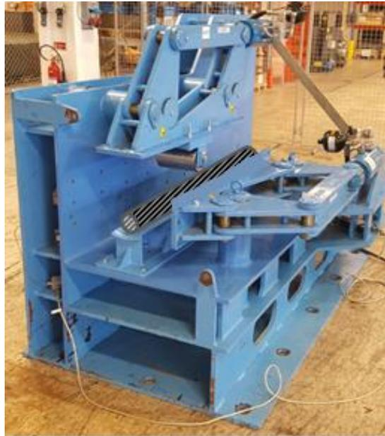
*Figure 3.25 - A double armoured cable in the squeeze rig.*
