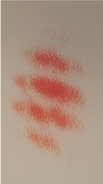
Figure 4.2 - Pressure distribution on the armouring wires
