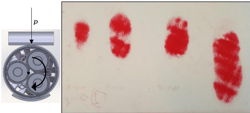
Figure 5.6 - Rotating of the cable during the loading will increase the larger ellipse diameter.
