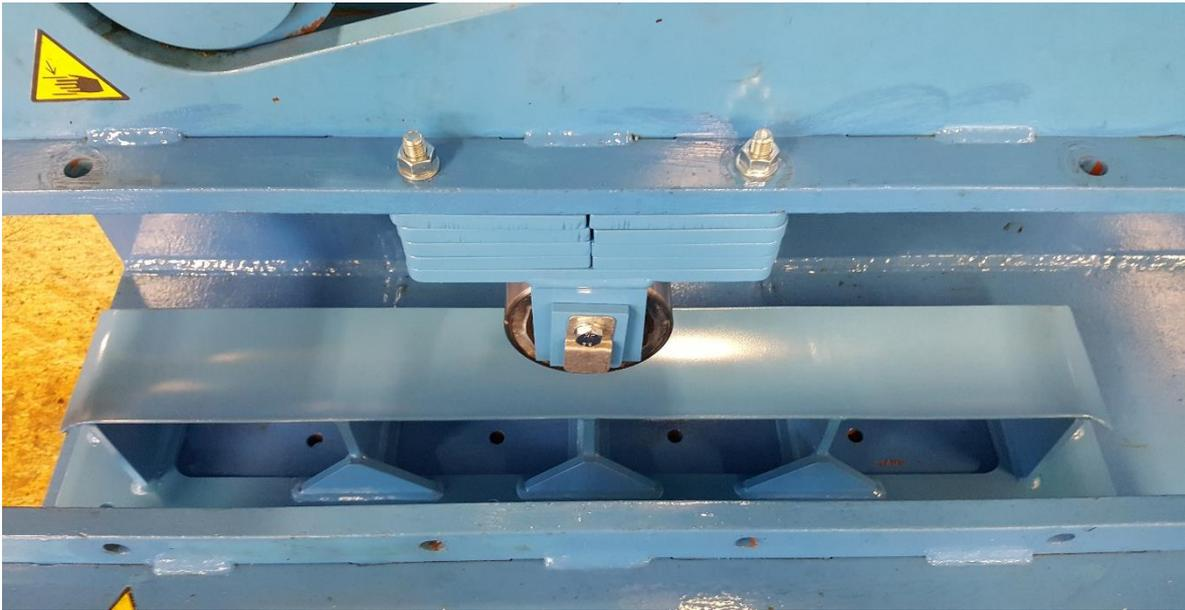
Figure 3.24 - Roller support mounted in the middle of the Squeeze rig's clamp.
