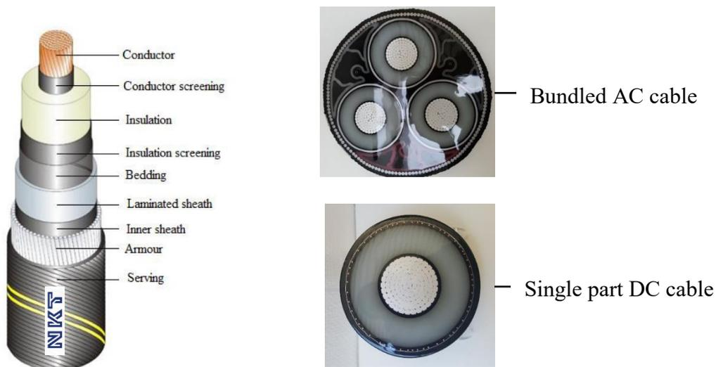
*Figure 1.1 - Cable compositions and cable types.*
