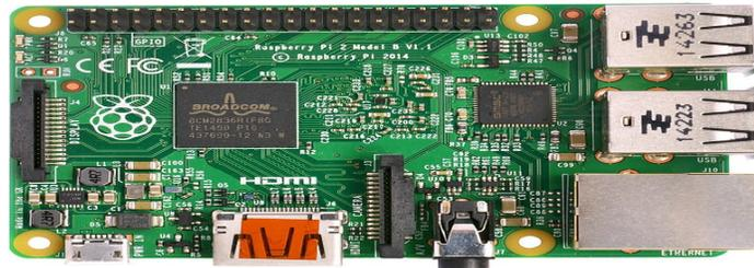
Fig. 1. A photo of raspberry pi board
