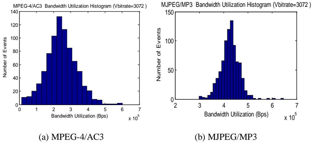
**Figure 5.14:** Bandwidth Utilization plots for MPEG-4/AC3 and MJPEG/MP3 codecs at 3072 kbps bit rate.
