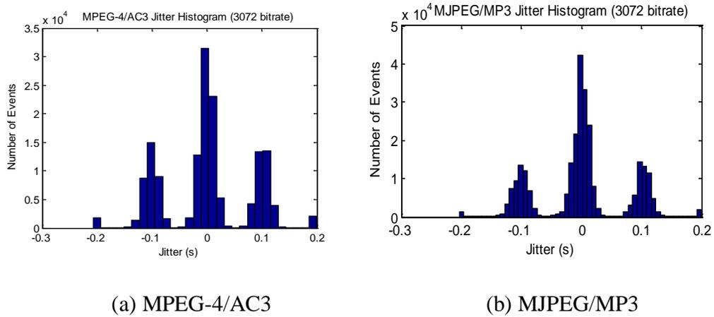
**Figure 5.10:** Jitter histograms for MPEG-4/AC3 and MJPEG/MP3 codecs at 3072 kbps bit rate.
