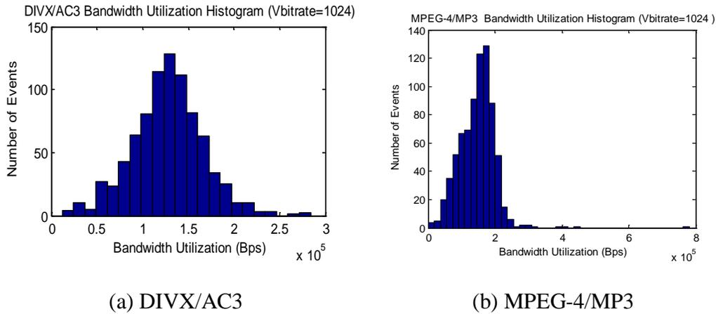
**Figure 5.8:** *Bandwidth Utilization plots for DIVX/AC3 and MPEG-4/MP3 codecs at 1024 kbps bit rate.*
