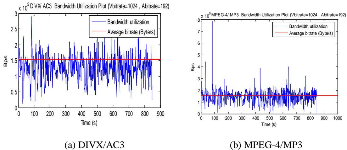
**Figure 5.7:** Bandwidth Utilization plots for DIVX/AC3 and MPEG-4/MPEG3 codecs at 1024 kbps bit rate.
