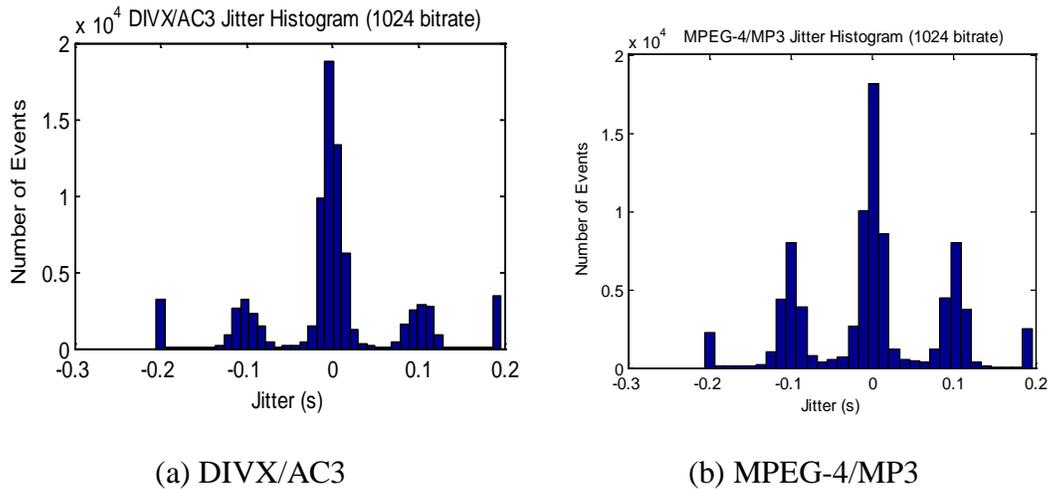
**Figure 5.3:** Jitter histograms for MPEG-4/MP3 and DIVX/AC3 codecs at 1024 kbps bit rate.
