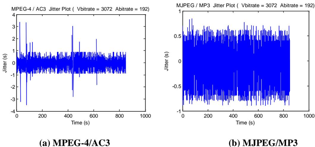
*Figure 5.9:* Jitter plots for MPEG-4/AC3 and MJPEG/MP3 codecs at 3072 kbps bit rate.
