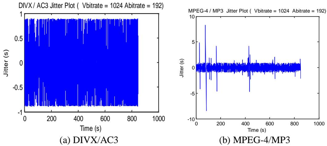
**Figure 5.2:** Jitter plots for DIVX/AC3 and MPEG-4/MP3 codecs at 1024 kbps bit rate.
