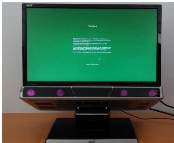
**Figure 3:** Shows the Asus VG248QE (in black) attached on top of the Tobii TX300 (in grey). The monitor was attached to the eye-tracker through a static stand to keep it fixated. The four purple lights visible in the figure are the IR-lights used to create the reflection in the eye.
