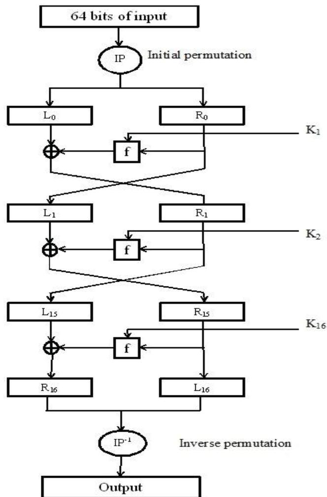
Fig2.2: DES Encryption Algorithm
