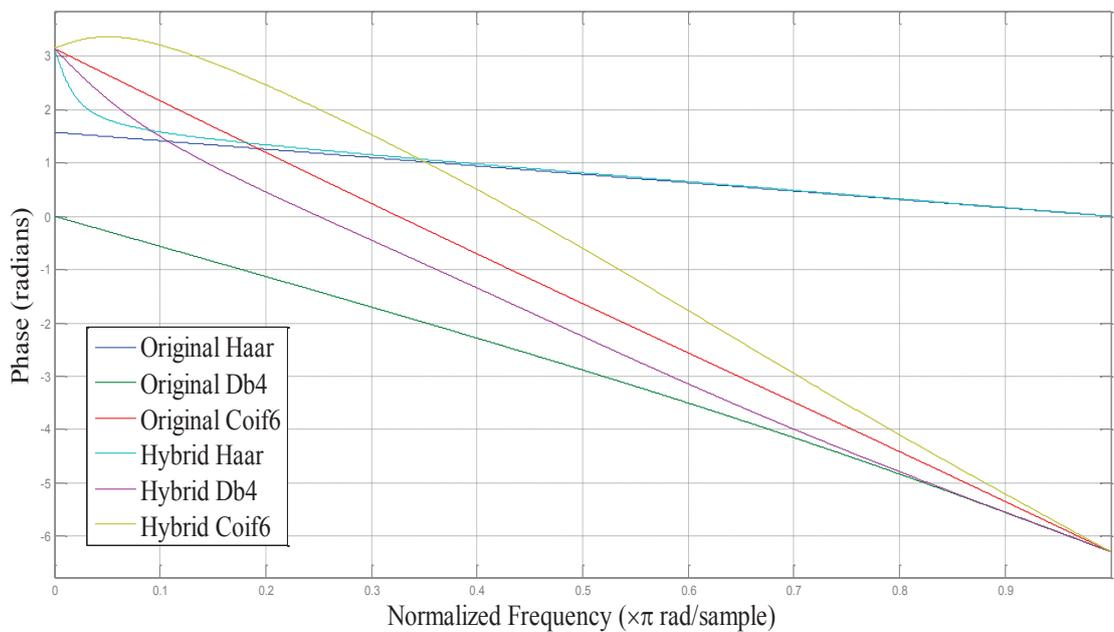
Fig 4.11: Phases of frequency response functions for original and hybrid Haar, Daubechies 4 and Coiflet 6 wavelets.
