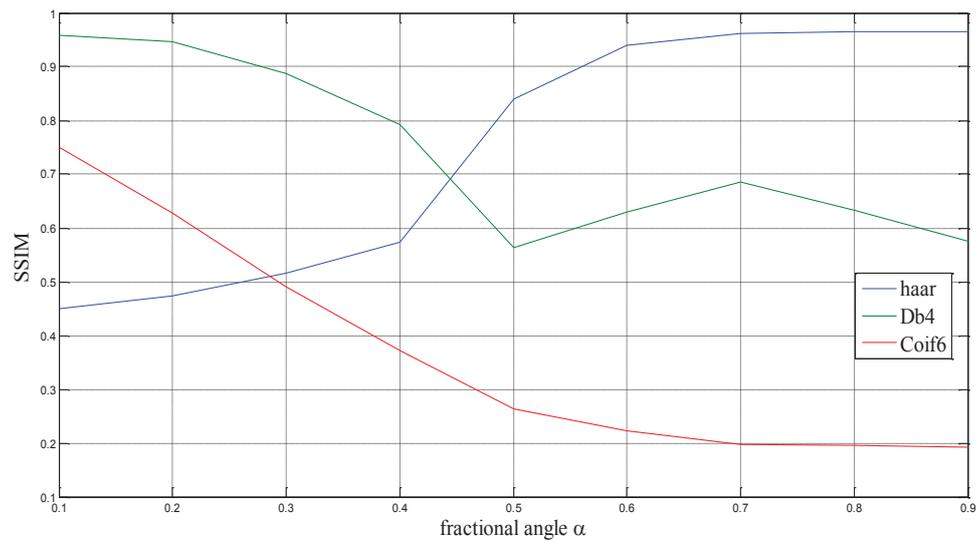
Fig 4.17: SSIM values for the reconstructed image of size 128x128 plotted against the fractional angle for hybrid Haar, Daubechies 4 and Coiflet 6 wavelets
