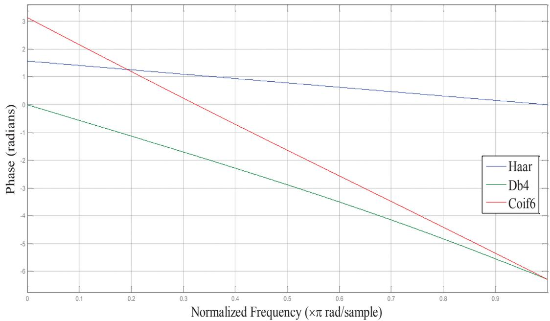
Fig 4.6: Phases of frequency response functions for Haar, Daubechies 4 and Coiflet 6 wavelets.
