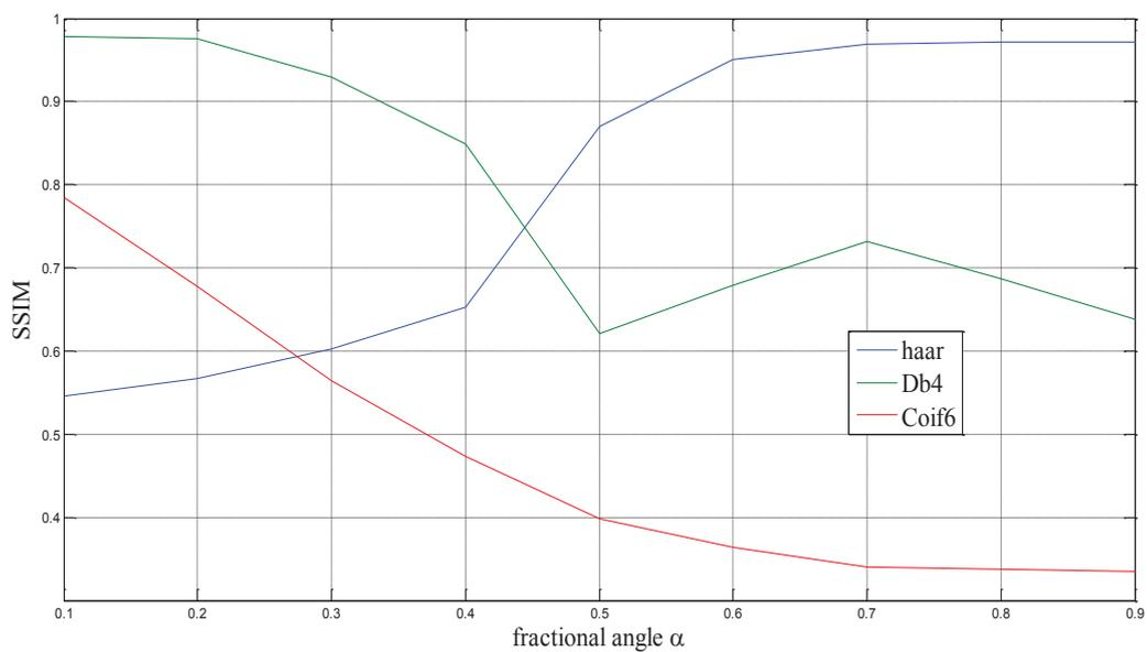
Fig 4.15: SSIM values for the reconstructed image plotted against the fractional angle for hybrid Haar, Daubechies 4 and Coiflet 6 wavelets
