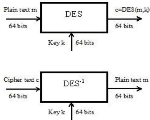
Fig2.1: DES Encryption and Decryption Algorithm
