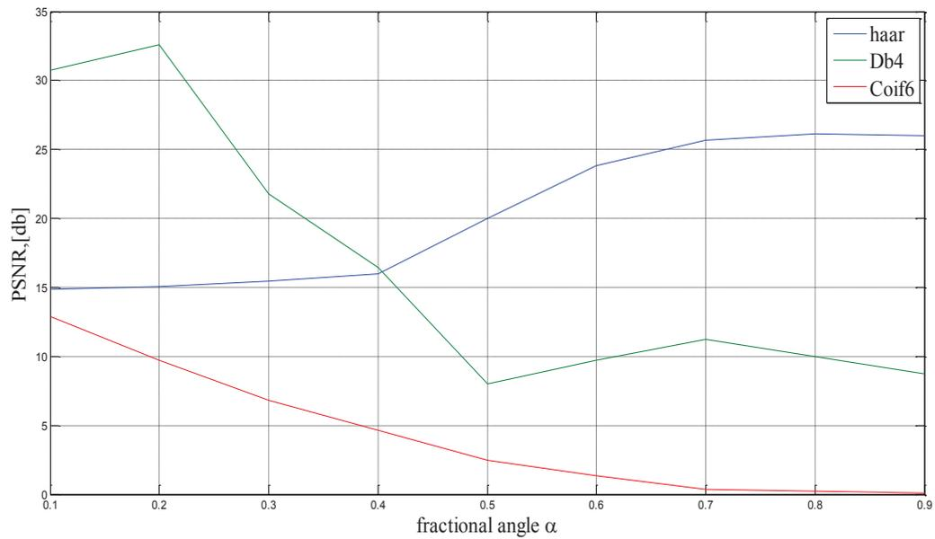
Fig 4.14: PSNR values for the reconstructed image plotted against the fractional angle for hybrid Haar, Daubechies 4 and Coiflet 6 wavelets
