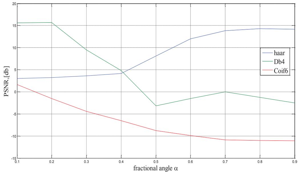
Fig 4.18: PSNR values for the reconstructed image of size 64x64 plotted against the fractional angle for hybrid Haar, Daubechies 4 and Coiflet 6 wavelets
