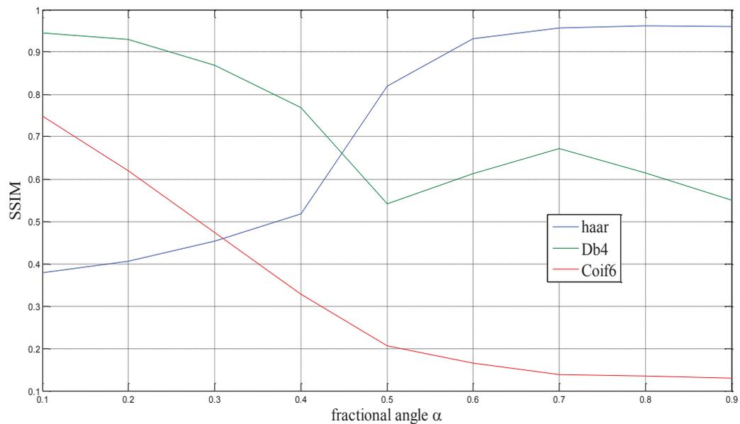
Fig 4.19: SSIM values for the reconstructed image of size 64x64 plotted against the fractional angle for hybrid Haar, Daubechies 4 and Coiflet 6 wavelets
