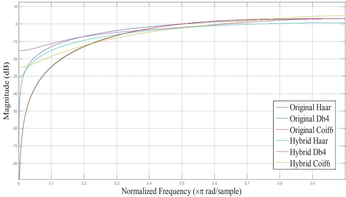
Fig 4.10: Magnitudes of frequency response functions for original and hybrid Haar, Daubechies 4 and Coiflet 6 wavelets.
