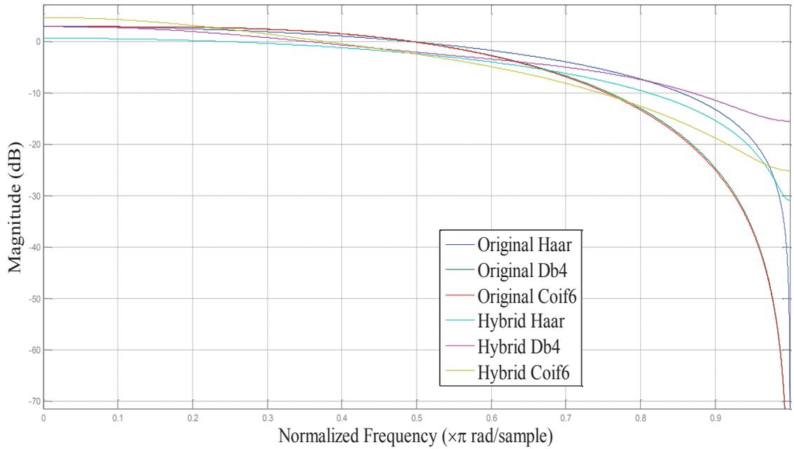
Fig 4.8: Magnitudes of frequency response functions for original and hybrid Haar, Daubechies 4 and Coiflet 6 wavelets.
