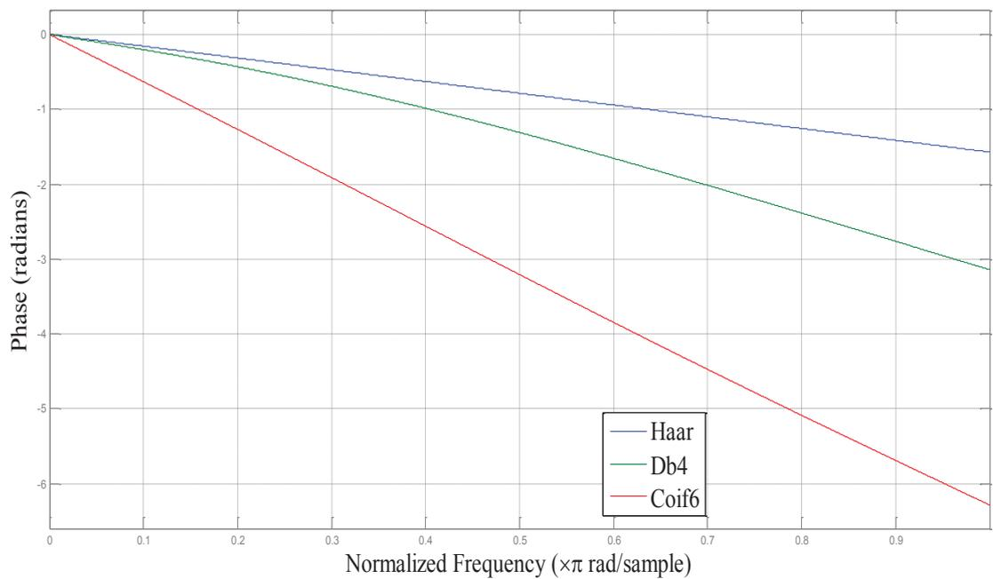
Fig 4.4: Phases of frequency response functions for Haar, Daubechies 4 and Coiflet 6 wavelets.
