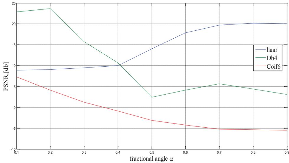
Fig 4.16: PSNR values for the reconstructed image of size 128x128 plotted against the fractional angle for hybrid Haar, Daubechies 4 and Coiflet 6 wavelets
