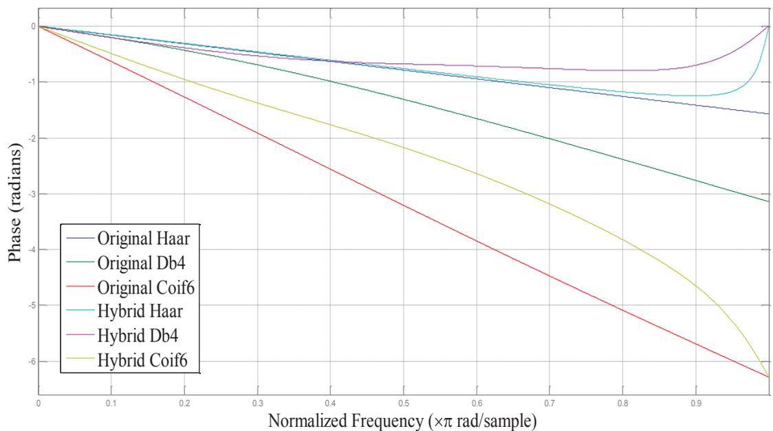
Fig 4.9: Phases of frequency response functions for original and hybrid Haar, Daubechies 4 and Coiflet 6 wavelets.
