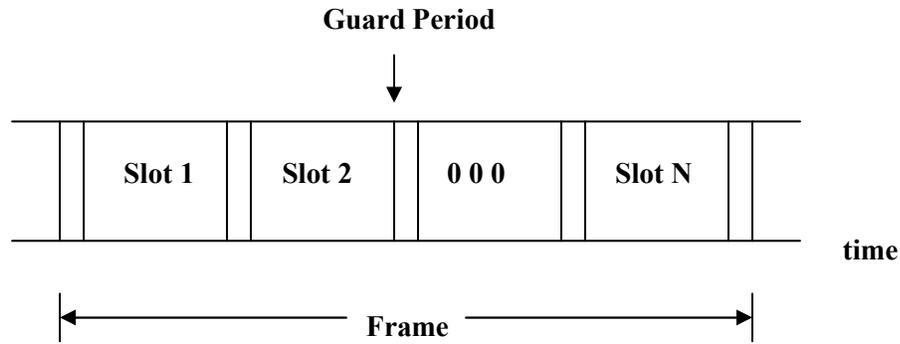
**Figure 1.2 TDMA frames Structure [1].**
