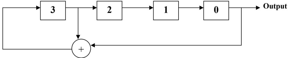
Figure 2.15 Multistage shift register to generate a PN codes [3]
