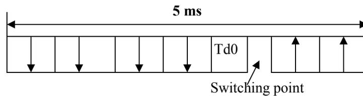
Figure 2.8 Asymmetric DL/UL Allocation [5]
