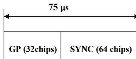
Figure 2.10 Burst structure of DwPTS [8]
