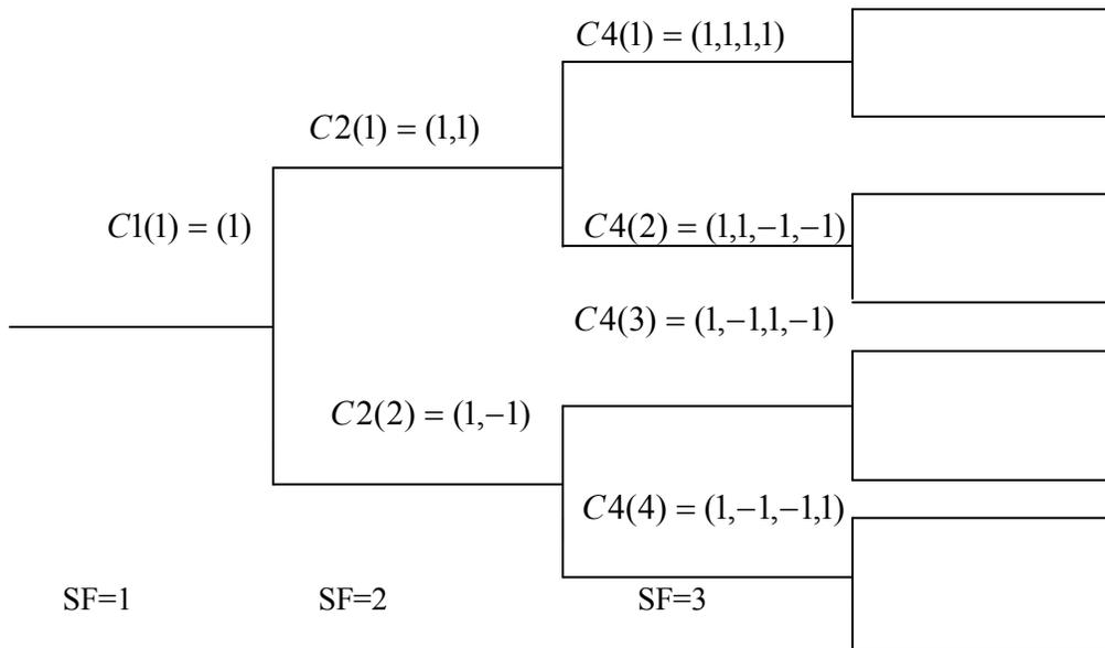
**Figure 2.13 Code-Tree for Generation of OVFSF [3]**
