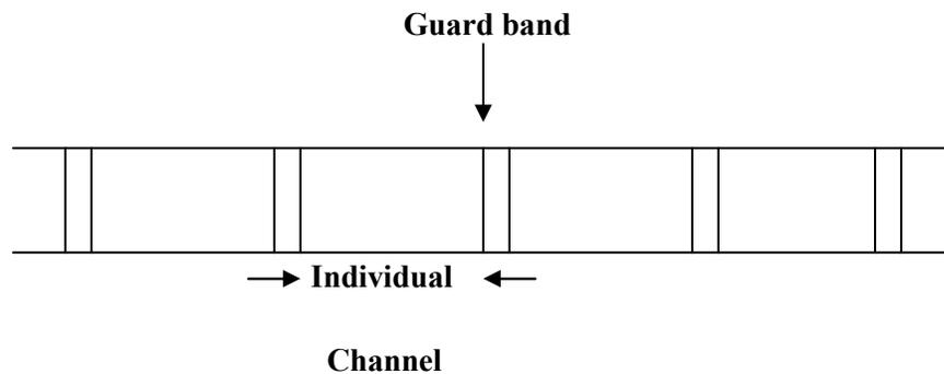
Figure 1.1 FDMA bandwidth spectrum [1].
