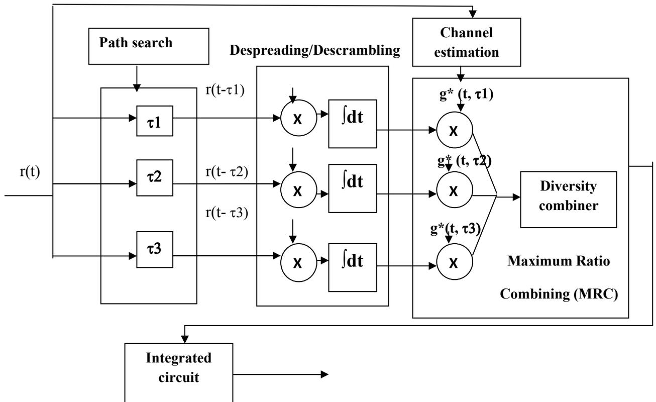
Figure 2.16 Rake receiver supported by TDD-CDMA [11]
