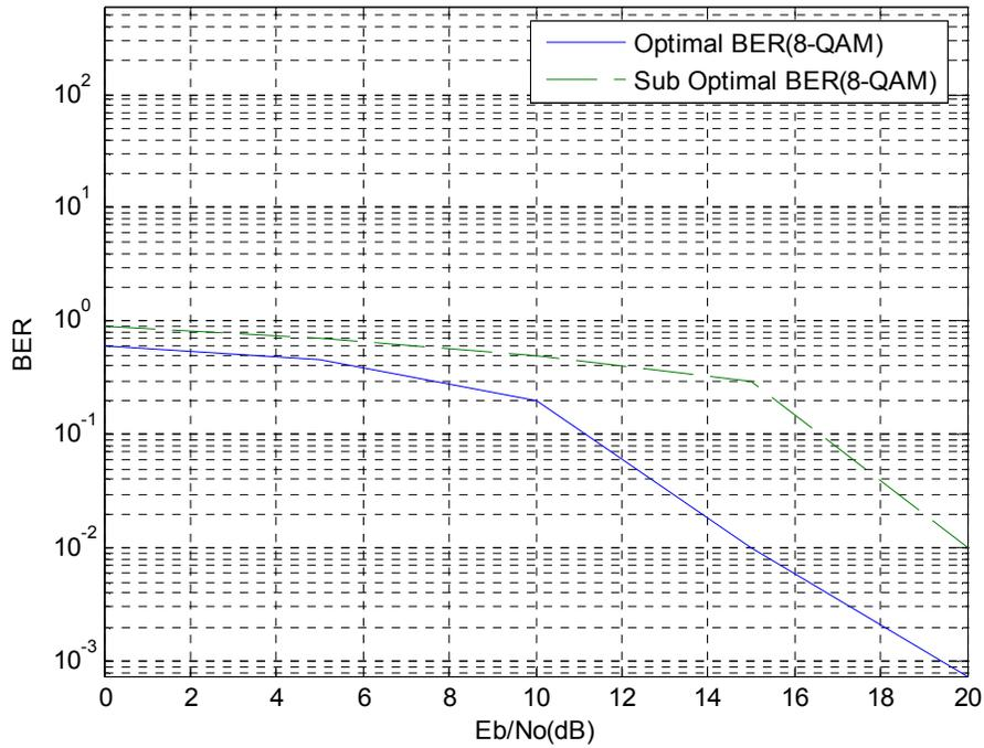
**Figure 5.9 Optimal and Sub Optimal Receiver in 8-QAM**
