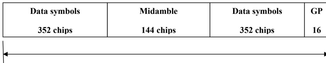
Figure 2.9 TD-SCDMA Slot Structure [7]
