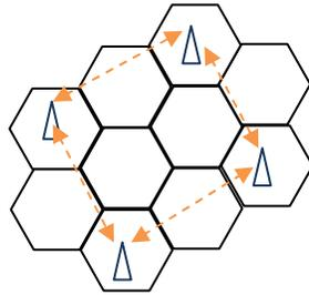
**Figure 3.7: Co-channel Interference Scenario [23]**
