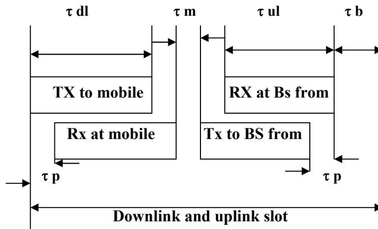
Figure 2.2 Uplink and downlink time slots [5]
