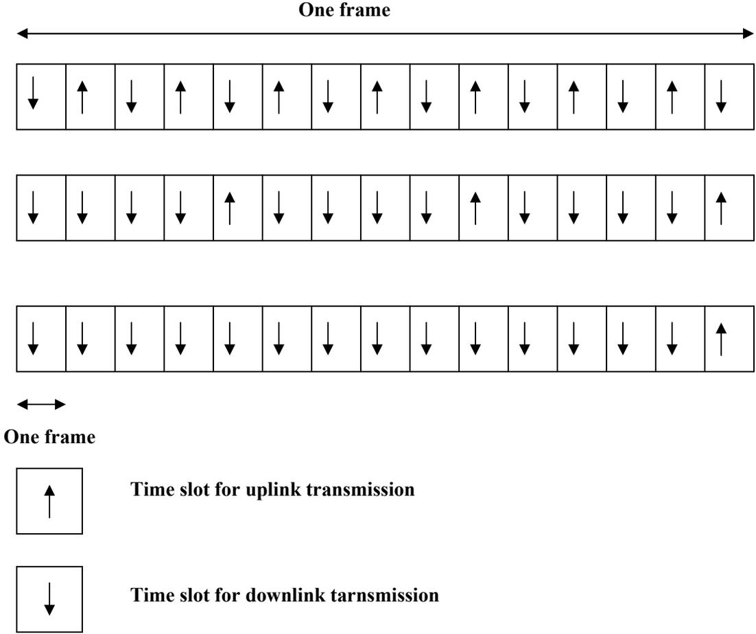
Figure 2.4 Number of Uplink and downlink time slots per frame [5].
