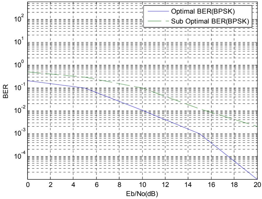
**Figure 5.7 Optimal and Sub Optimal Receiver in BPSK**
