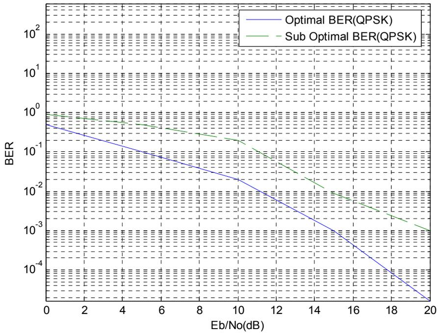
**Figure 5.8 Optimal and Sub Optimal Receiver in QPSK**
