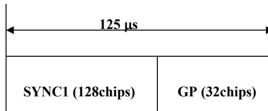
Figure 2.11 Burst structure of UpPTS [8]
