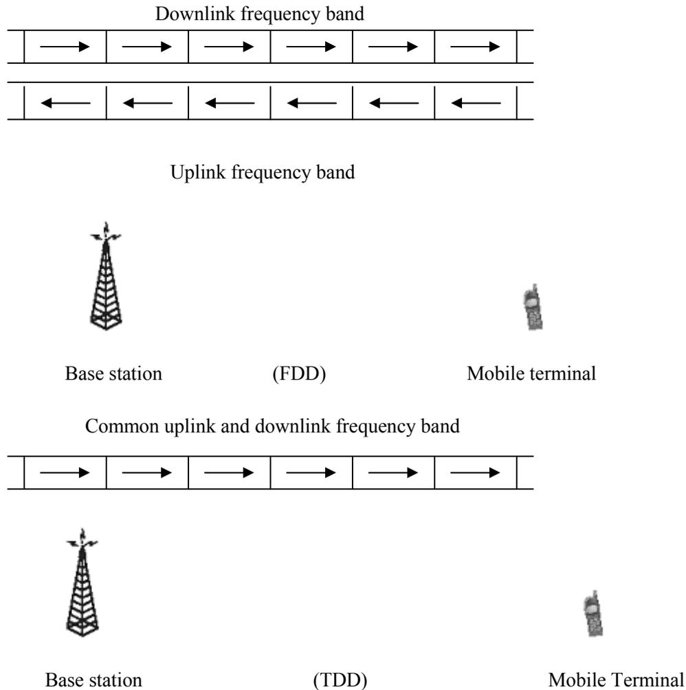
Figure 1.1 FDD and TDD duplexing mode [5]
