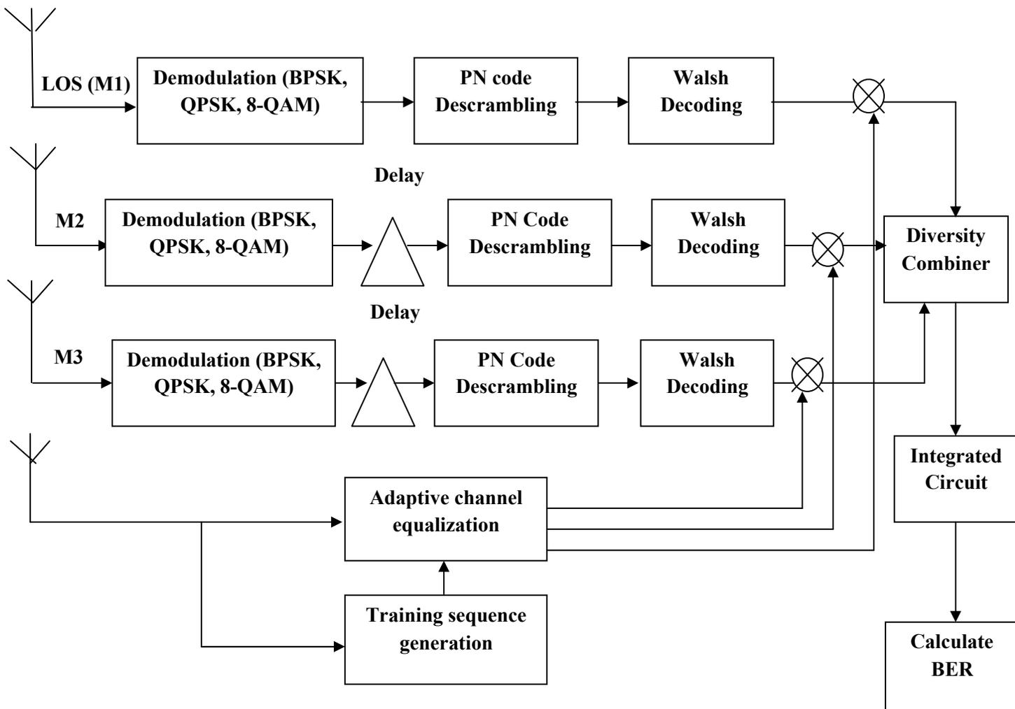
Figure 3.10.Receiver Module [11]
