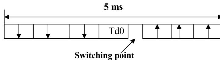
Figure 2.7 Symmetric DL/UL Allocation [5]
