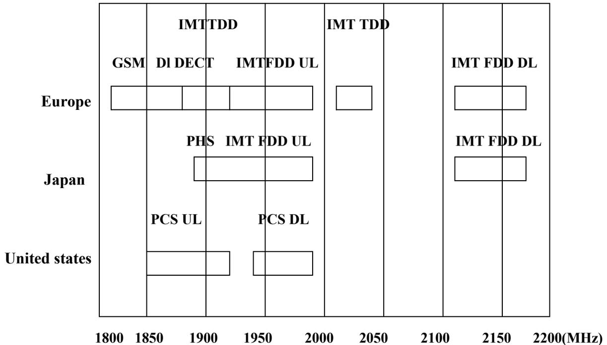
Figure 2.5 Frequency Plan [5]
