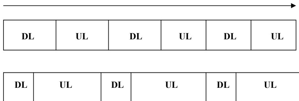
Figure 2.3 Unequal slot lengths [5]
