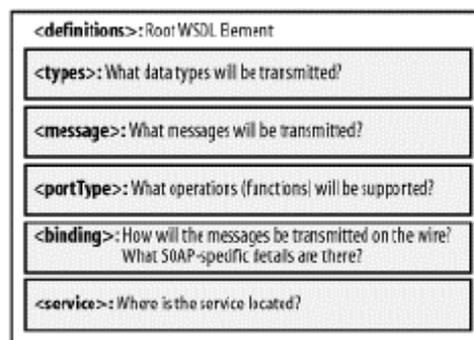
Figure 3 The WSDL Specification in a nutshell [8]
