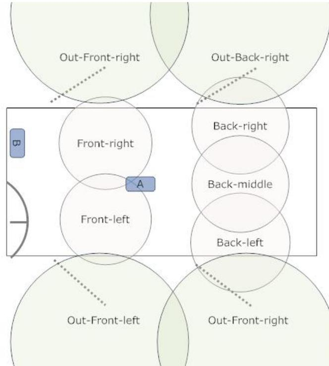
Fig. 5.11 Illustration of vehicle areas and proposed Bluei RFID reader placement
