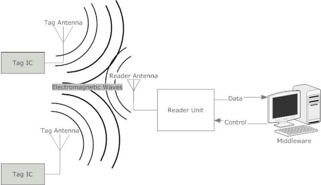
Fig. 2.1 Components of an RFID System
