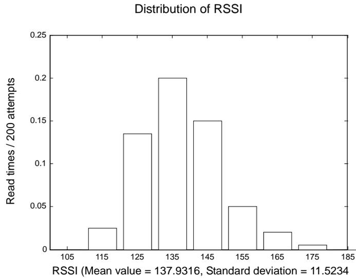
Fig. 6.1 Result of Test A.2 with Wavetrend active tag in out-front-left area
