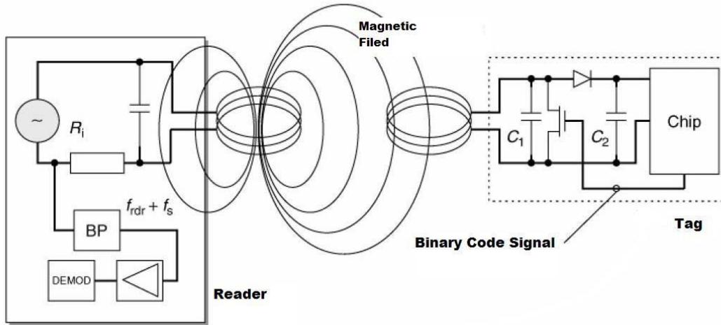
Fig 2.2 Near-filed Coupling
