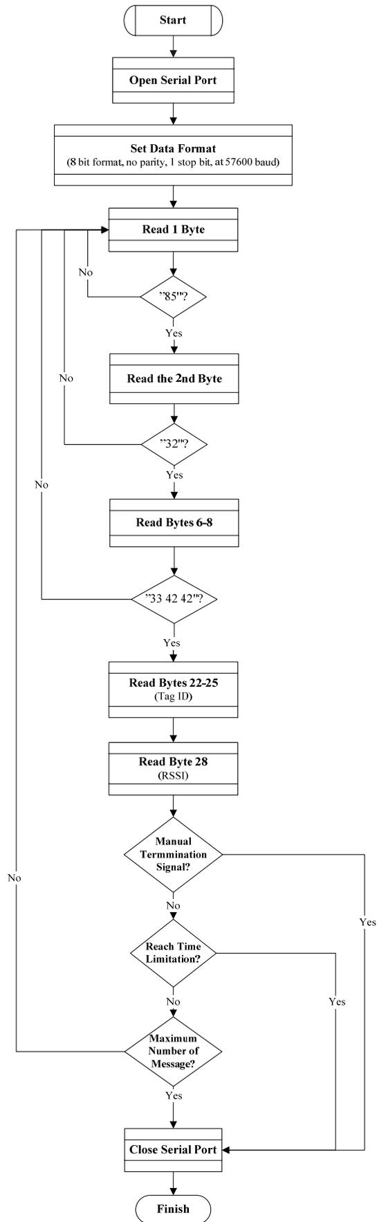
Fig.5.1 Flowchart of the C program (RFID\_tag\_read.c)
