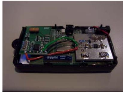
Fig. 5.3 Wavetrend L-TG501 active Tag and Bluei RFID Reader
