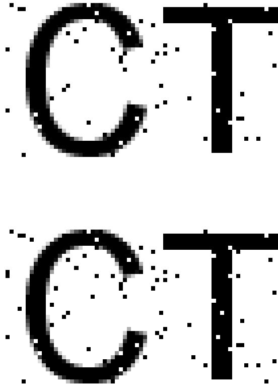
Figure 3.2: Enlarged excerpt from figure 3.1, showing the last two characters ("CT") from degradation iteration 6 (top) and 7 (bottom). Tesseract recognized the top image recognized as "CT", whereas the bottom image was recognized as "CLT"
