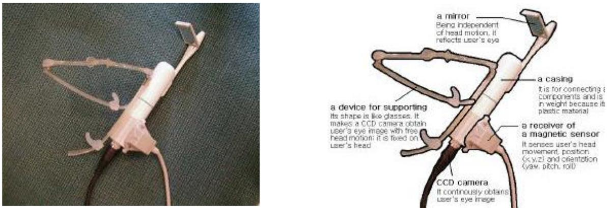
Figure 4.2: Head mounted eye Tracking System along CCD camera, [17]
