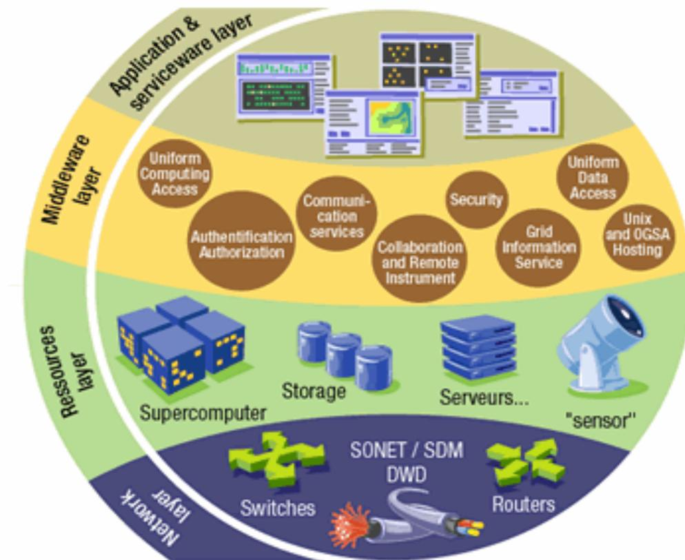
Figure 4.1: Layered Architecture of the Grid [17]
