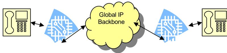
*Figure 6.3: Voice over IP system with computer enabled analogue to digital conversion*
