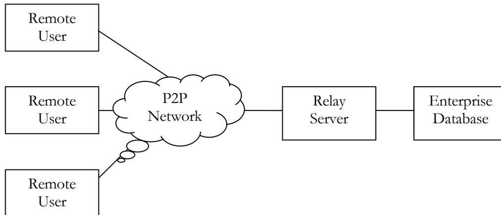
*Figure 4.8: A schematic representation of the Groove Networks architecture*
