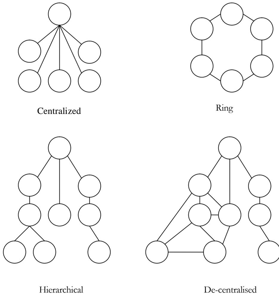
*Figure 2.3: A schematic representation of the basic network topologies that could be used in a P2P network*
