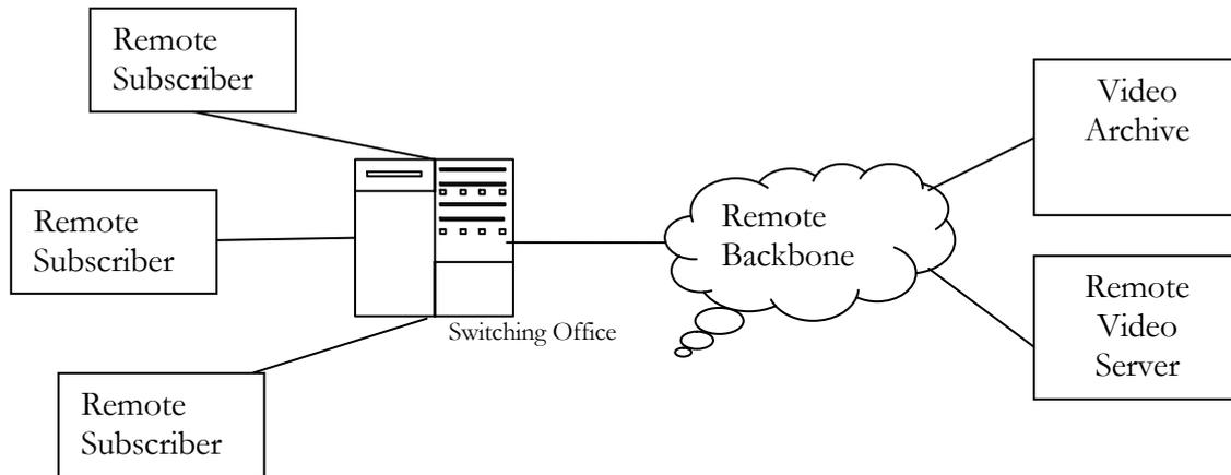
Figure 4.6: A representation of a Video on Demand Service Architecture
