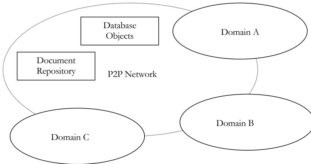
*Figure 4.9: A schematic representation of a Knowledge Database running on a P2P Network*
