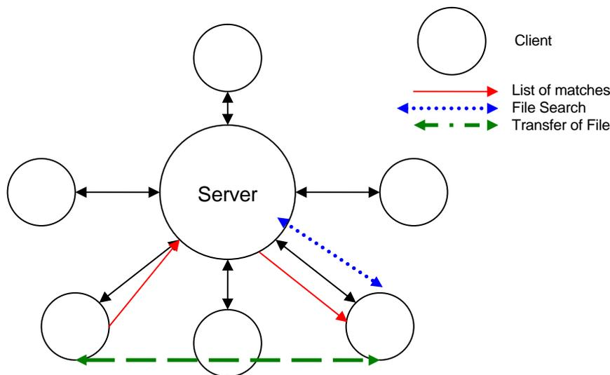
Figure 2.1: A Centralised P2P system with a server to facilitate data transfers
