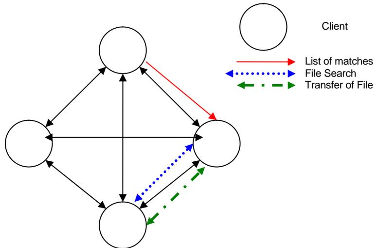
Figure 2.2: A De-centralised P2P system with peers directly connected to facilitate data transfers
