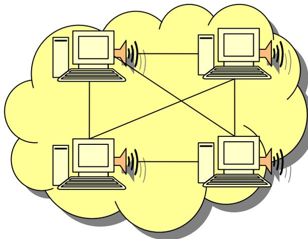
*Figure 6.4: Peer to Peer based Voice network running over the global IP network*
