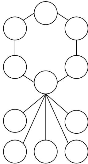
Figure 2.4: A representation of a Ring + Centralised combo network topology
