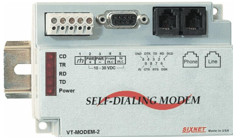
**Figure 19:** SIXNET PLC Self-dialing modem
