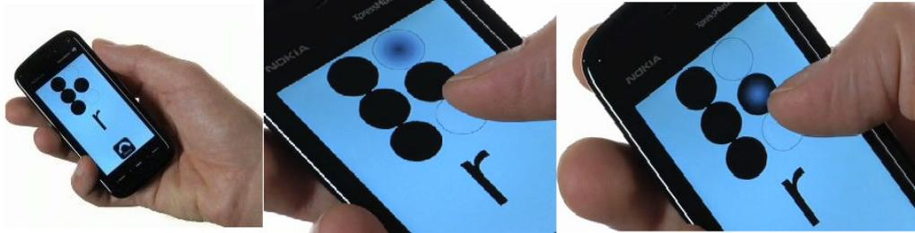
**Figure 5.7: Nokia Braille Reader: The user hold a finger on the screen and application read the cells dot by dot [29]**
