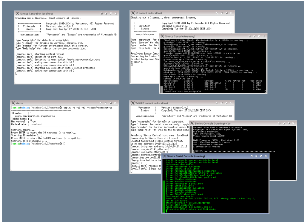
Figure 7.1: TSP cluster in Simics, consists of one IO machine (upper right window), one TelORB machine with its serial console also visible (lower right window), and a Simics Central instance (upper left window). The cluster has been started from the lower left console window.
