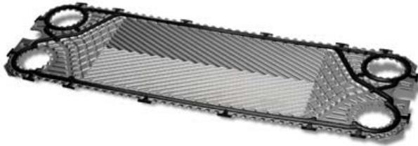
Plate heat exchangers are usually designed to achieve turbulence across the entire heat transfer area in order to get the highest possible heat transfer coefficient with the lowest possible pressure drop, and allow for close temperature approach. Consequently this means smaller heat transfer area, smaller heat exchangers, and sometimes even less heat exchangers [1].
