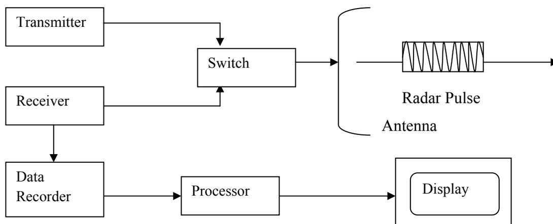
Fig. 2.1: Basic block diagram of typical radar system.
