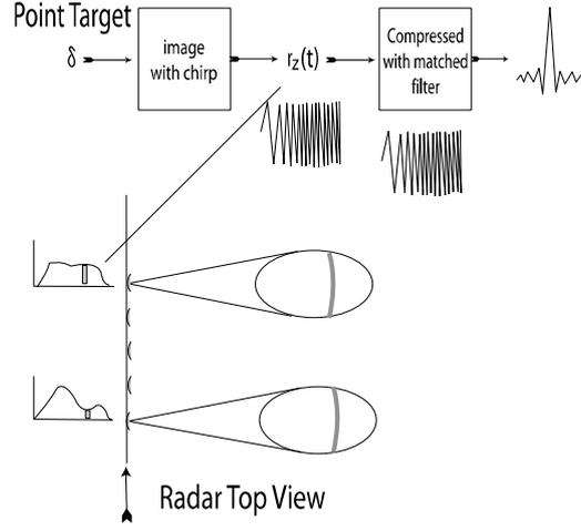
Fig 2.5: Match filtering of received echo [11].
