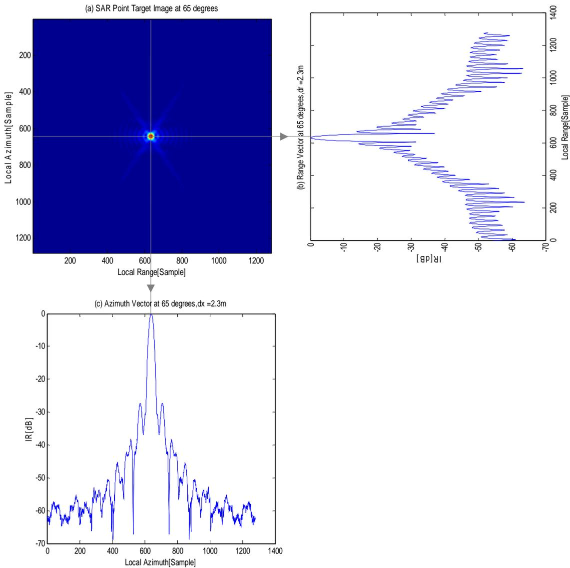
Fig. 6.1: (a) A point target is imaged by an UWB SAR system with an integration angle of 65 degrees, (b) The extracted range vector from the peak, (c) The extracted azimuth vector from the peak.
