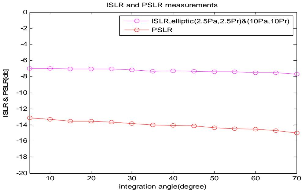
Fig 6.6: ISLR and PSLR at different integration angles.
