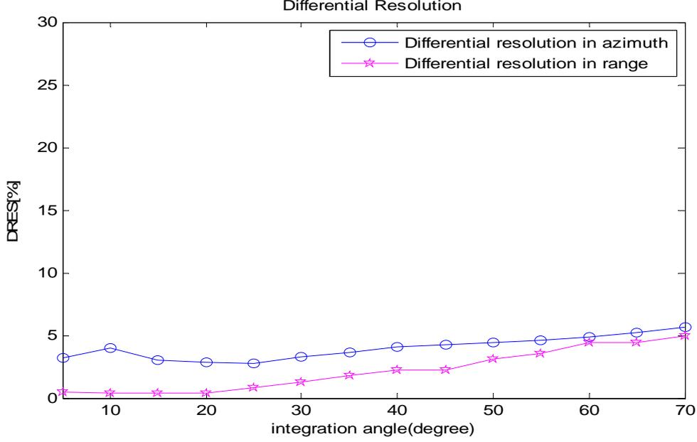
Fig 6.3: Plot of the differential resolution calculations.
