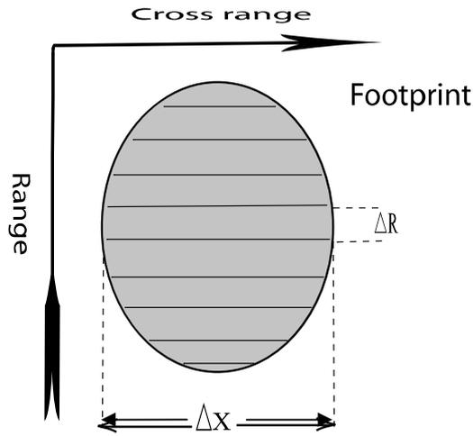
Fig. 2.4: Cross-range and range resolution of SAR [3].
