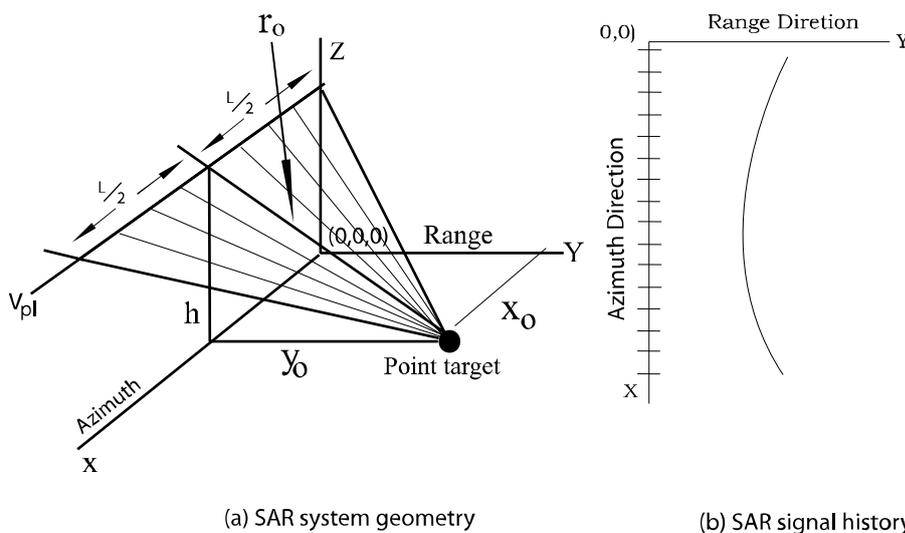
Fig. 3.2: (a) SAR system geometry and (b) SAR signal history.
