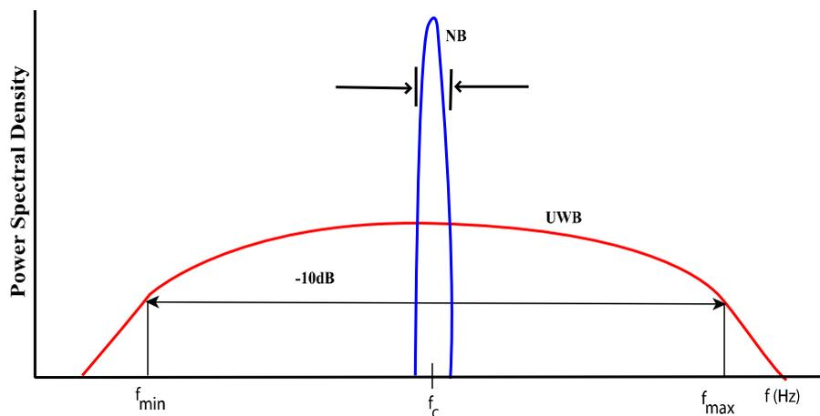
Fig. 2.6: Power spectral density of NB and UWB signals.
