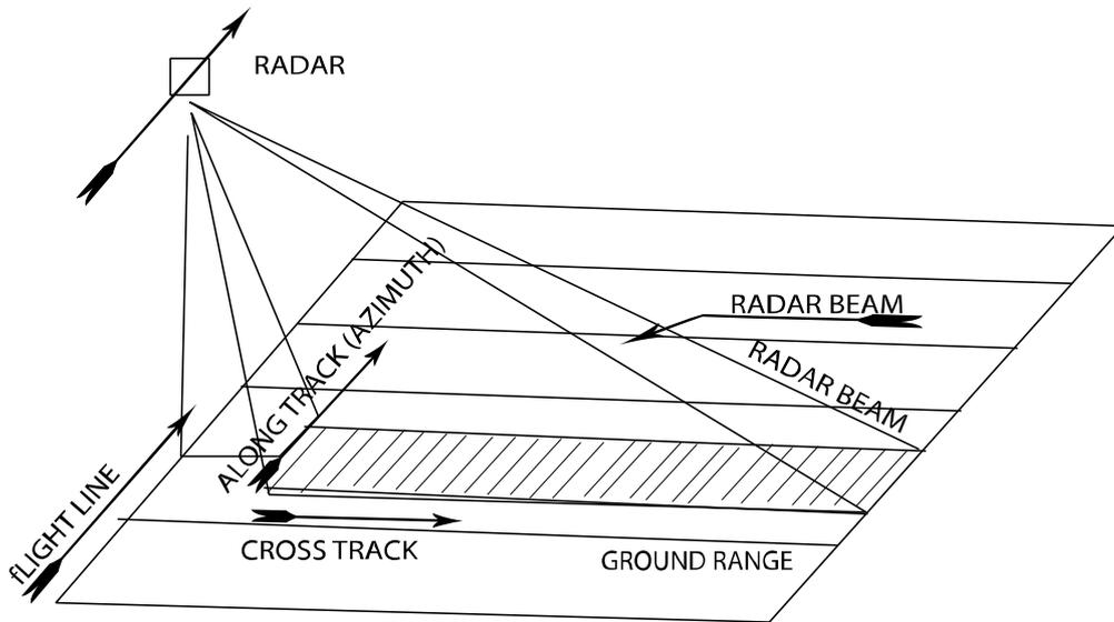
Fig. 2.3: SAR geometry.
