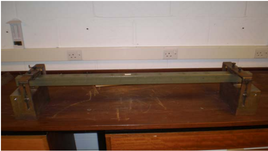
Figure 5.12: Beam position on fixed-fixed position
