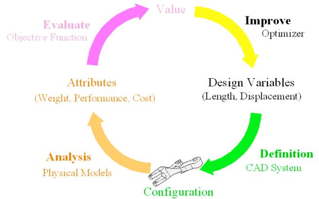
Figure 1: The Value Driven Design cycle [11]
