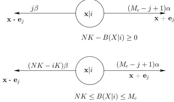
**Figure 4.3:** The state diagram of a one dimension CTMC with buffering
