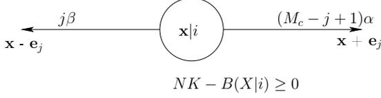
**Figure 4.2:** The state diagram for a one dimension CTMC without buffering
