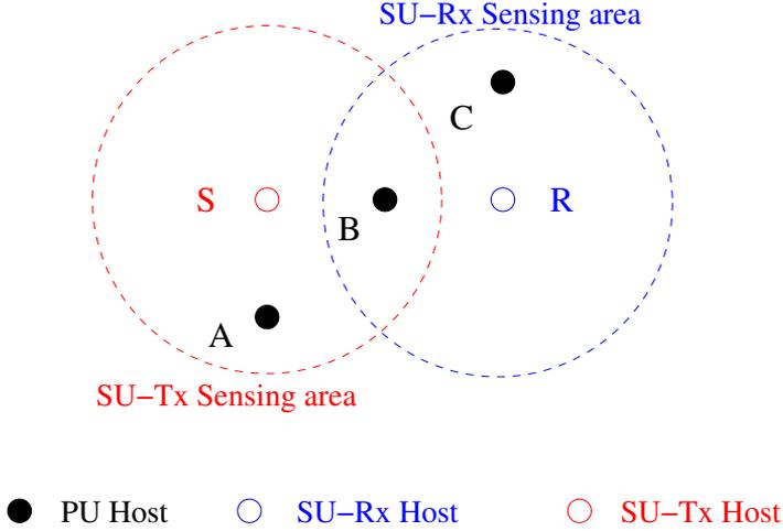
**Figure 2.1:** *Illustration of a cognitive radio channel*
