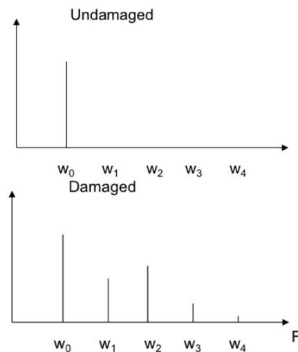
Figure 1. When a single frequency is input to the material, the same frequency is measured when the material is undamaged, top. When the material is damaged, higher harmonics are created, below.
