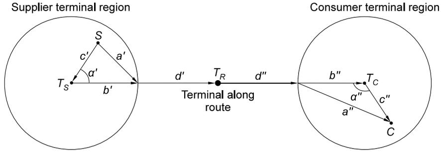
Fig. 2: Illustration of distances for different routes from a supplier  $S$ , via a terminal  $T_R$  to a consumer  $C$ . Transportation may occur, e.g., via terminals  $T_S$  and  $T_C$  ( $c' + b' + d' + d'' + b'' + c''$ ) or direct by road ( $a' + d' + d'' + a''$ ).
