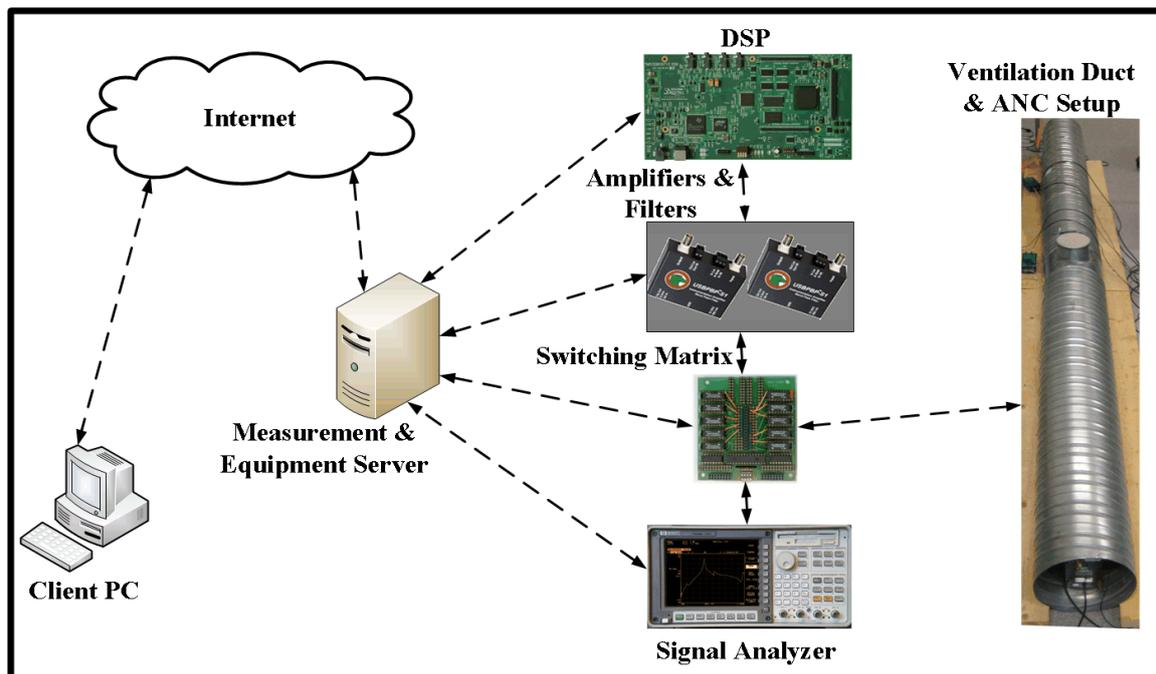
Figure 1. Block diagram of the remotely controlled ANC system.
