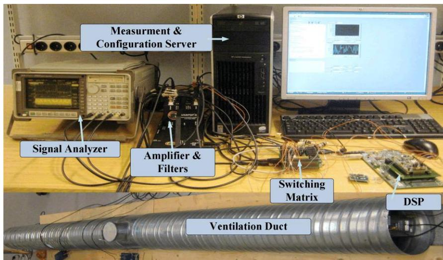
Figure 2. Remote ANC Laboratory hardware setup.
