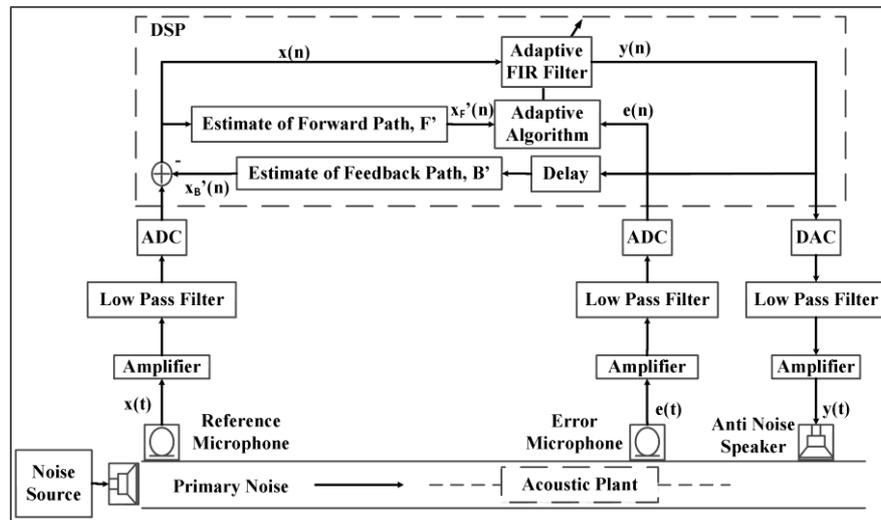
Figure 4. Schematic diagram for a single channel feed forward ANC system in the remote ANC lab.
