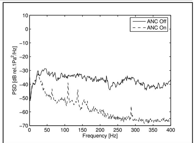
**Figure 5.** Power spectral density (PSD) of the error microphone signal with the reference and error microphones placed in microphone boxes based on T-duct. Solid line shows the ANC system off, and dashed line shows the ANC system on.
