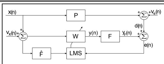
Figure 2. Block diagram of the filtered-x LMS algorithm with measurement noise at the reference- and error sensors,  $v_x(n)$  and  $v_e(n)$ , respectively.
