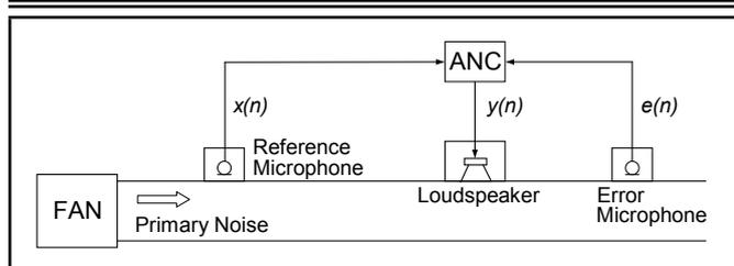
Figure 1. Single-channel feedforward ANC system applied to a duct.
