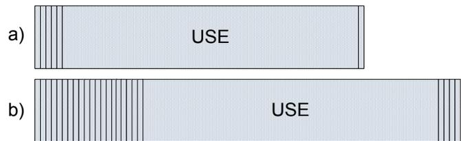
Figure 5: Environmental impact comparison between one long-life light tube (top) and three standard-life light-tubes (bottom). Vertical bars represent the life cycle stages in Figure 4. Top bar shows the long-life product, with 1/4 of impacts from stages other than use, compared to bottom bar that shows standard-life product. Impacts from use phase are the same for both.
