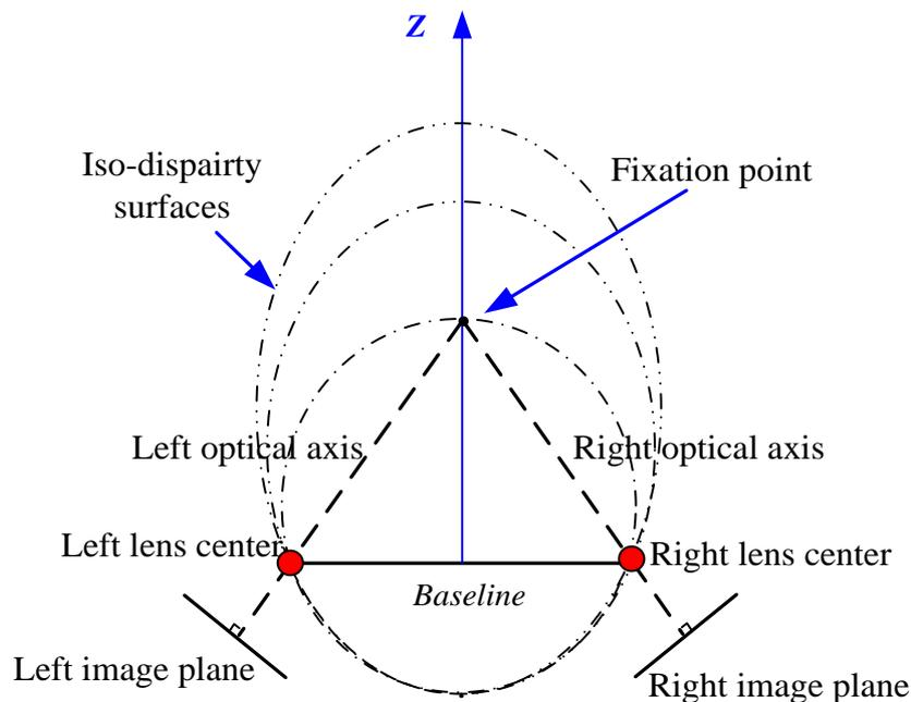
Figure 3.2. An illustration of the iso-disparity surfaces' geometry model for the convergent stereo pair in the plane defined by the cameras' optical axes.
