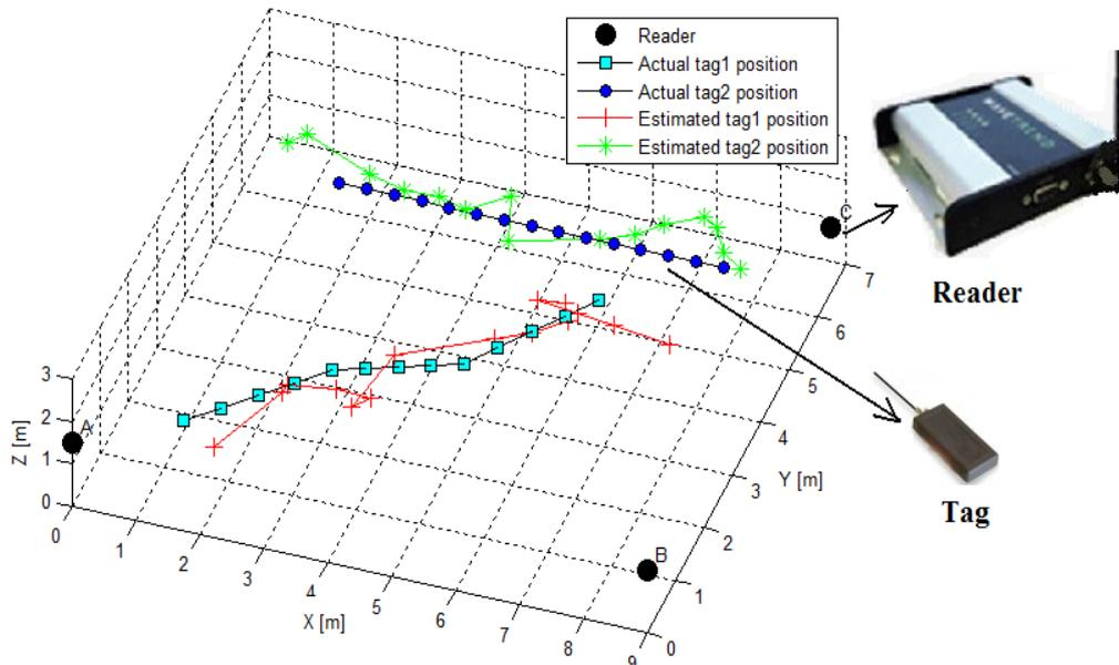
Fig. 4. The schematic diagram of the physical experiment
