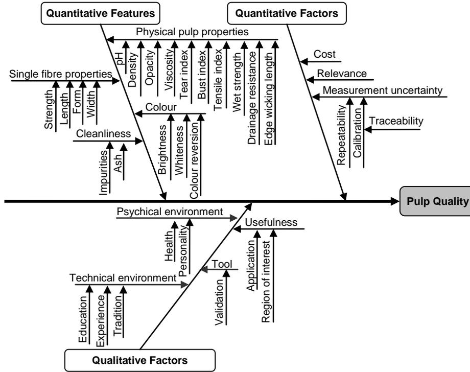
Fig. 9. Definition of the pulp quality modelled by the Ishikawa diagram.
