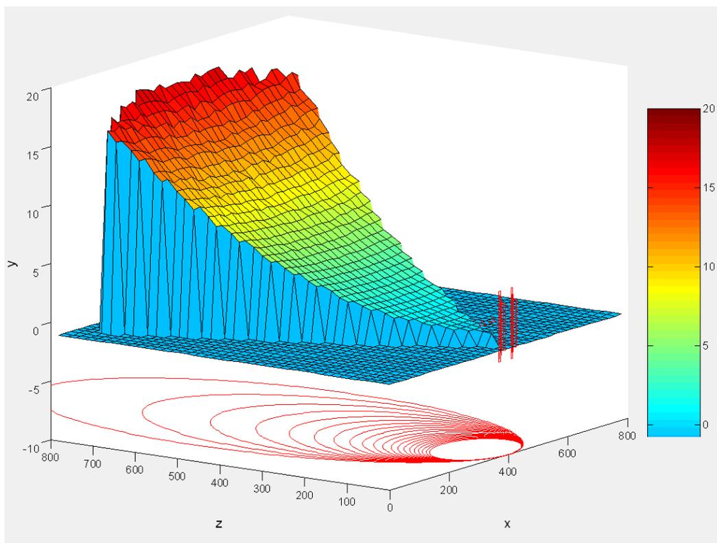
Fig. 4. The depth reconstruction uncertainty map for a stereo pair's FoV, where  $B=40$  cm,  $f=3.5$  cm,  $p=0.004$  cm.
