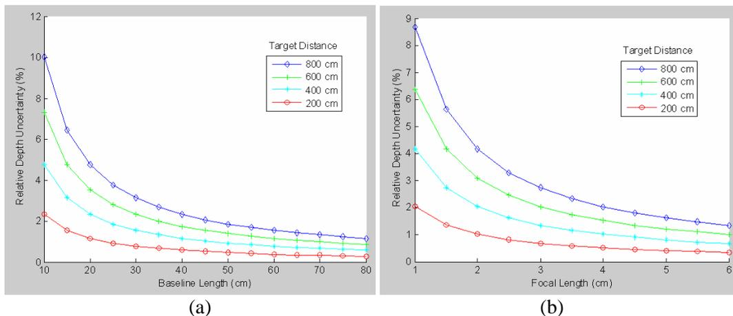
Fig. 6. The uncertainty varies with the baseline length, focal length, sensor pixel length, and stereo convergence angle. The distance from the target to the camera is 800 cm, 600 cm, 400 cm and 200 cm, respectively. They are marked by different type of lines. The uncertainty varies with (a) the baseline length; (b) the focal length.
