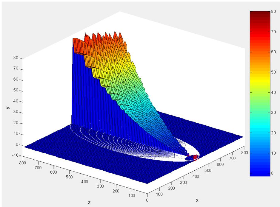
Fig. 5. The depth reconstruction uncertainty map for a stereo pair's half FoV, where  $B=20$  cm,  $f=3.5$  cm,  $p=0.008$  cm.
