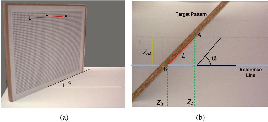
Figure 5.2. The target grid position: (a) front view, (b) top view.
