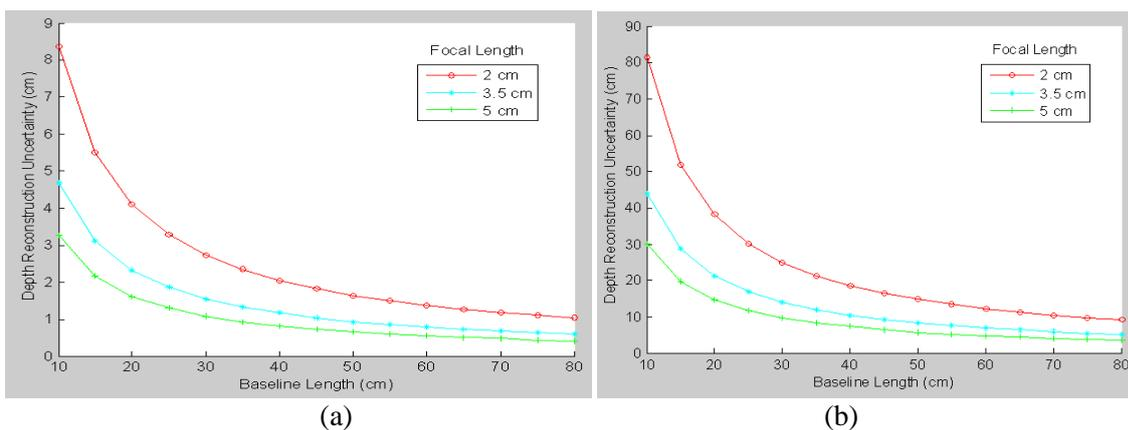
Fig. 8. The uncertainty varies with both the focal length and the baseline length. The focal lengths are 2 cm, 3.5 cm and 5 cm, respectively, marked by different type of lines. The target is (a) 200 cm; (b) 600 cm faraway from the camera.
