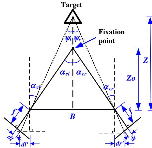
Fig. 1. The model of stereo pair geometry;  $Z_0$  is the depth of the fixation point,  $|dl-dr|$  is stereo disparity,  $f$  is focal length.
