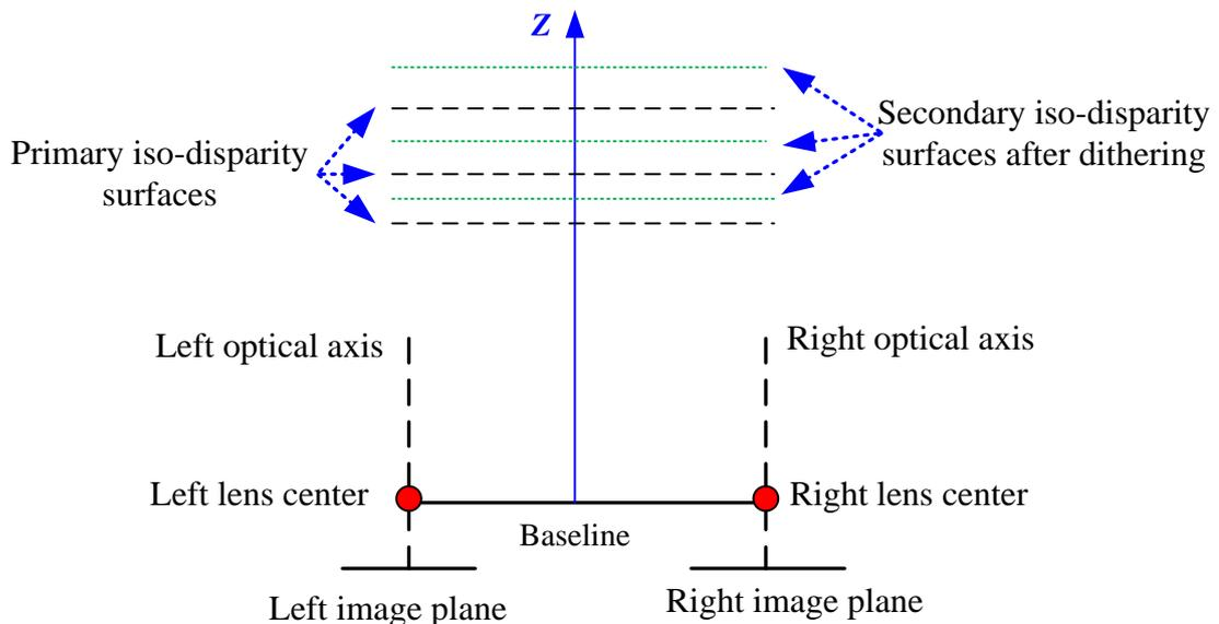
Figure 3.4. The combination of primary and secondary iso-disparity surfaces for the parallel stereo pair in the plane defined by the cameras' optical axes.
