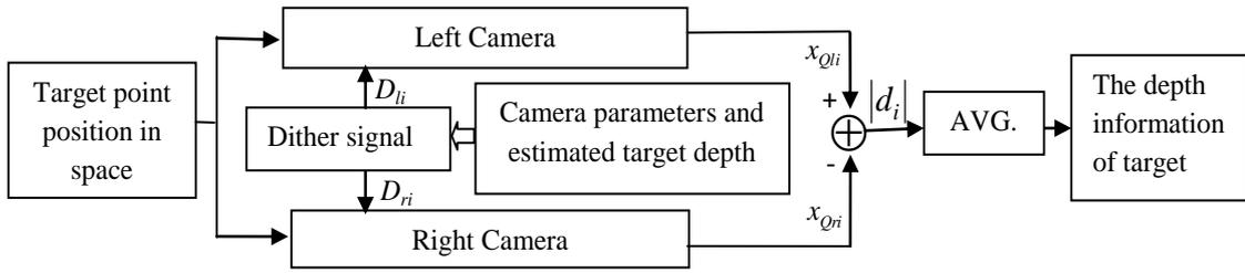
Fig. 5. The block diagram of the dithering algorithm where  $D_{li}$  and  $D_{ri}$  are the dither signals for the left and right cameras,  $x_{Qli}$  and  $x_{Qri}$  are the quantized signals for the left and right cameras, and  $d_i$  is disparity.
