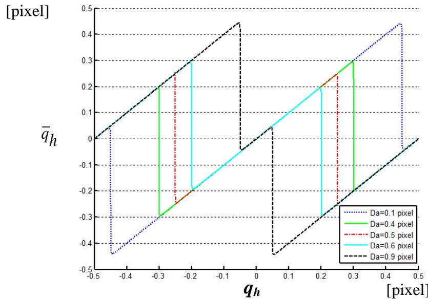
Fig. 2. The mean image horizontal quantization uncertainty with the dither signal,  $\bar{q}_h$ , versus the image horizontal quantization uncertainty  $q_h$  for different amplitude values of the dither signal amplitude  $D_a$ .
