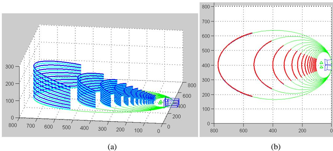
Fig. 3. Simulation results of iso-disparity surfaces for a stereo pair from the synthetic model (bold red line) and mathematical model from equation (4) (green line) with convergence angle,  $\alpha_c=4^\circ$ , the baseline length  $B=40$  cm, the focal lengths  $f=2.5$  cm and disparity resolution  $\Delta D=0.04$  cm (a) perspective view, and (b) top view.
