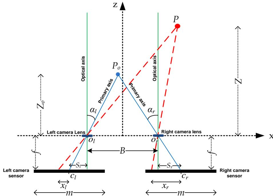
Fig. 1. An  $x$ - $z$  view of the skewed-parallel stereo camera schematic diagram.
