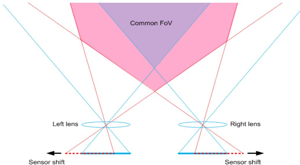
Figure 3.3. The common FoV where the blue solid lines represent the parallel stereo setup and the red dashed lines represent the parallel sensor-shifted stereo setup. Shaded areas are the common FoV for the parallel and sensor-shifted stereo setups respectively.
