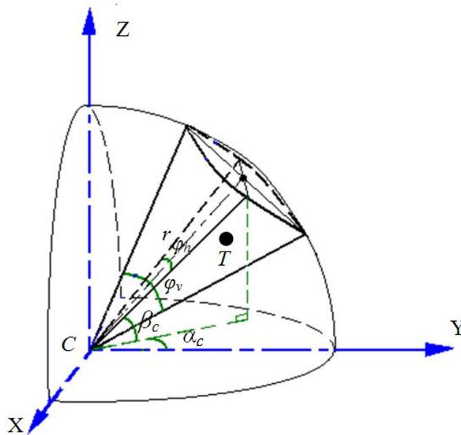
Figure 4.2. The spherical coordinate system and FoV of a camera where  $C$  is the camera position and the example target point is located at the point  $T$ .
