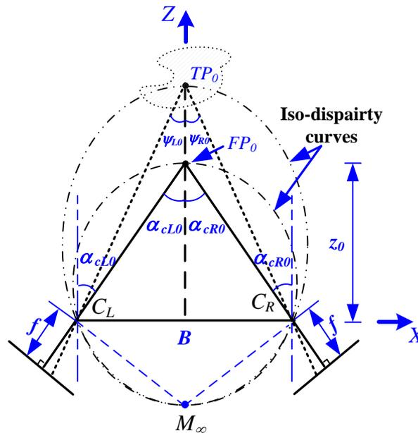
Fig. 2. An example of the iso-disparity curves for the convergence stereo pair in the plane defined by the cameras optical axes.  $z_0$  is the distance from the fixation point to the baseline,  $f$  is the focal length.
