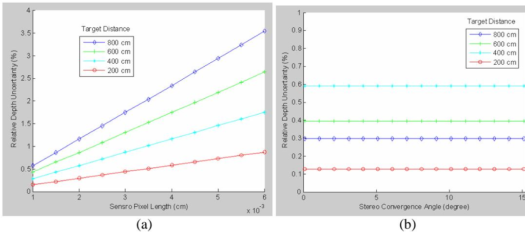
Fig. 7. The uncertainty varies with the baseline length, focal length, sensor pixel length, and stereo convergence angle. The distance from the target to the camera is 800 cm, 600 cm, 400 cm and 200 cm, respectively. They are marked by different type of lines. The uncertainty varies with (a) the sensor pixel sizes; (b) the convergence angle.
