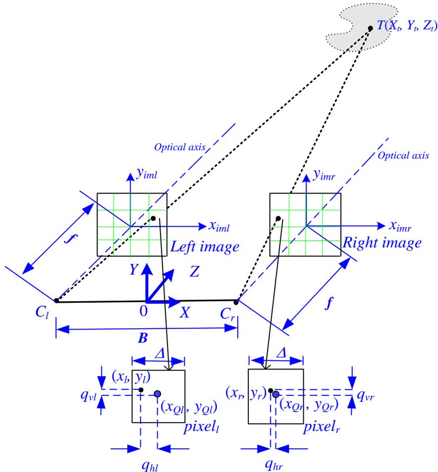
Fig. 1. Parallel stereo pair geometry and the image quantization uncertainty model.
