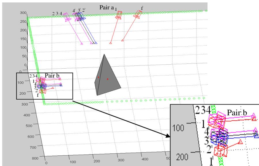
Fig. 3. The stereo pair positions and baseline lengths for the same target location vary according to the different accuracy.
