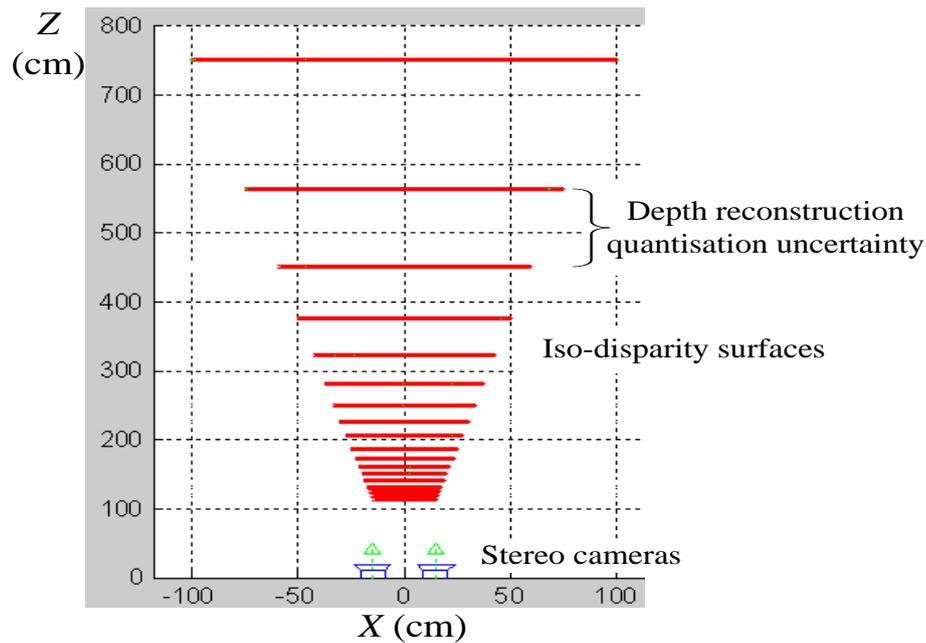
Figure 3.5. The depth reconstruction quantisation uncertainty is represented as the interval between the iso-disparity surfaces.
