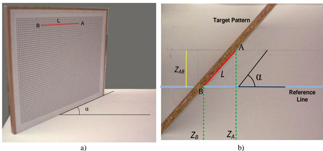
Fig. 7. The target grid positioning: a) front view, b) top view.
