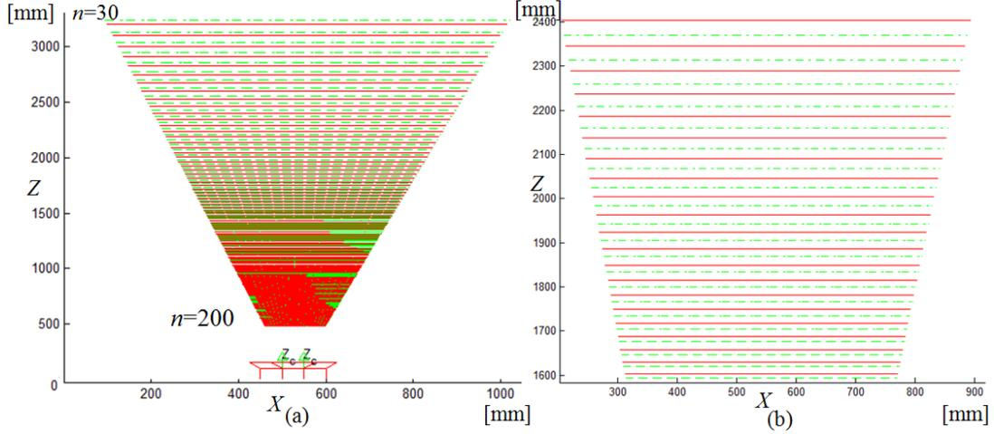
Fig. 3. (a) The iso-disparity planes for parallel cameras where  $\Delta = 12.9 \mu\text{m}$ , and  $f = 25 \text{ mm}$ ; the red solid lines for  $B = 50 \text{ mm}$ , the green dashed lines for  $B = 50.51 \text{ mm}$ . (b) The zoomed iso-disparity planes for  $Z_n$  were in the range from 1600 mm to 2400 mm.
