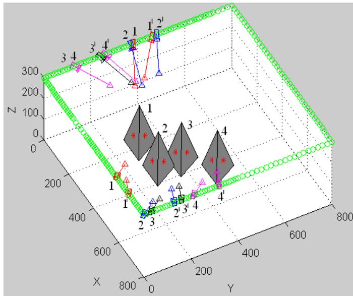
Fig. 2. The stereo pair positions, poses and baselines with the depth accuracy factor  $AF_{con} = 8$ , for the moving target.
