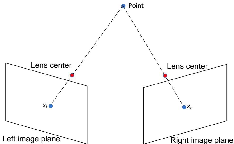
Figure 3.1. The point in 3D space can be reconstructed by a triangulation method.
