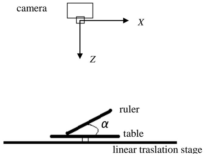
Fig.8. The photo and schematic diagram of objects and configurations in the physical experiment.
