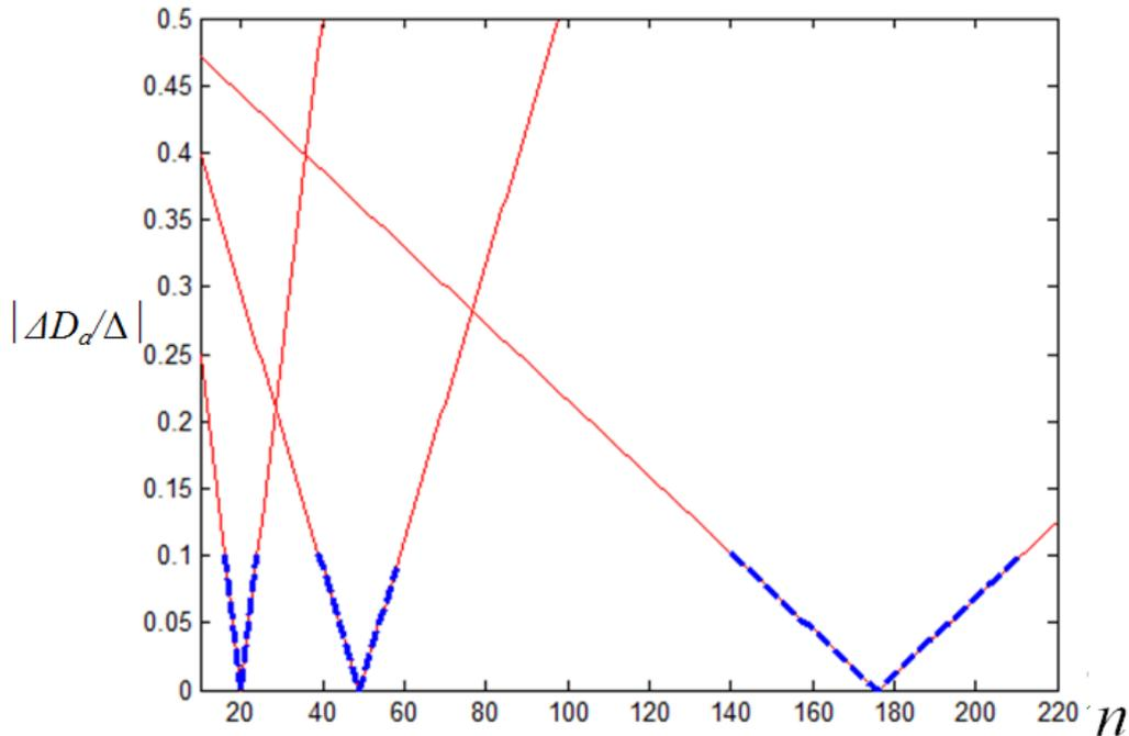
Fig. 4. The normalized deviation of the projection displacement,  $|\Delta D_d/\Delta|$  represented by red solid lines, and  $|\Delta D_d/\Delta| \leq 0.1$  represented by blue dashed lines;  $n_t=20, 49$  and  $179$ , while  $\Delta=12.9 \mu\text{m}$ ,  $B=50$  mm and  $f=25$  mm.
