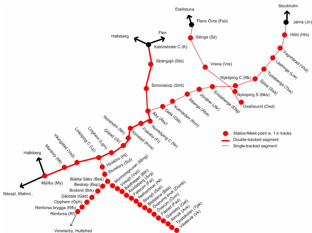
Figure 3. The railway (sub-)network used for the scenarios and corresponding experiments. Stations and sidings are connected by one or several segments that are either single- or double-tracked. Segments that are stations or other meet points can be  $n$ -tracked, i.e. have  $n$  parallel tracks.
