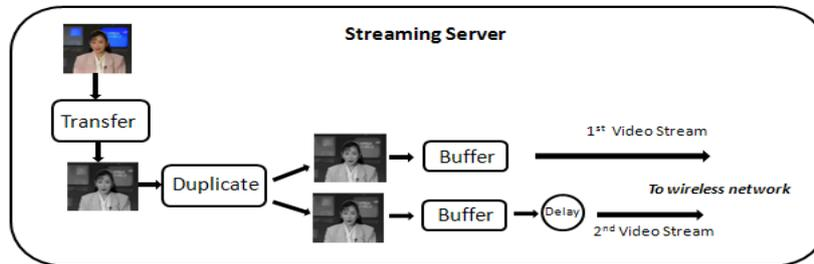
Figure 1. Streaming duplicate frames over two wireless channels.
