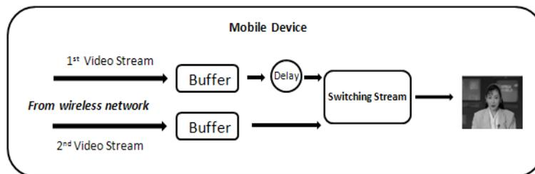
Figure 2. Receiving duplicate streams of video in the same mobile device.
