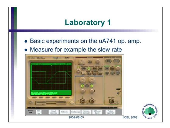
The oscilloscope is showing a typical result when measuring the slew rate.
