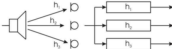
Figure 2: Schematic picture over multimicrophone system modelled as a single input multiple output system
