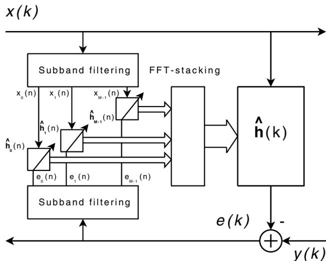
Figure 1: Closed loop delayless subband adaptive filtering configuration.
