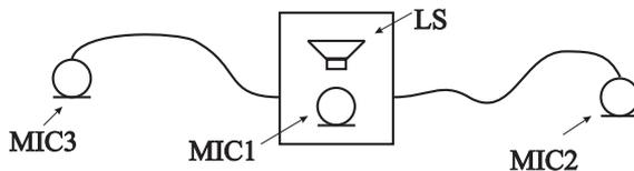
Figure 1: AEC unit with expansion microphones
