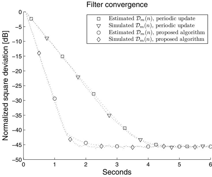
Figure 4: Comparison between the estimated and simulated squared deviation of the proposed methods and the periodic NLMS, respectively. Simulations were performed with an ideal setup, i.e. independent input samples and orthogonal filter coefficient vectors. Estimated deviations were obtained through equation (29) for the periodic updating scheme and equation (33) for the proposed algorithm.
