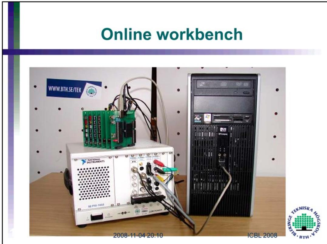
This is the online workbench. Where are the desktop instrument displayed on the client screen? They are replaced by PXI boards. PXI is a standard for instrumentation. The important thing is that the performance of the boards are equal or better than the performance of the desktop instruments.
