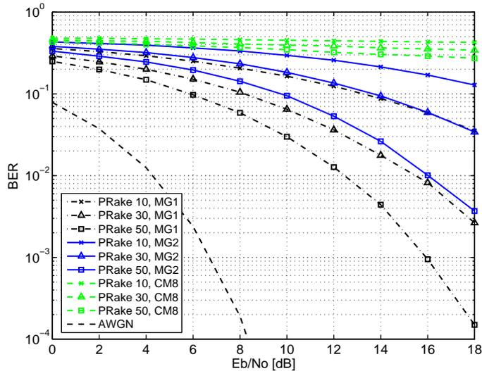
Figure 5.2: Comparison of BER of different number of fingers of PRake with MRC combining on MG1, MG2 and CM8.
