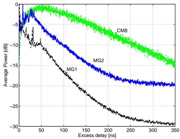
Figure 3.4: Average power delay profiles of MG1, MG2 and CM8 averaged over all channel realizations.
