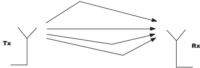
Figure 1.3: An illustration of multipath propagation over a wireless channel, where Tx and Rx stand for the transmitter and receiver, respectively.
