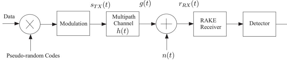
Figure 2.2: Block diagram of the system model (single-user).
