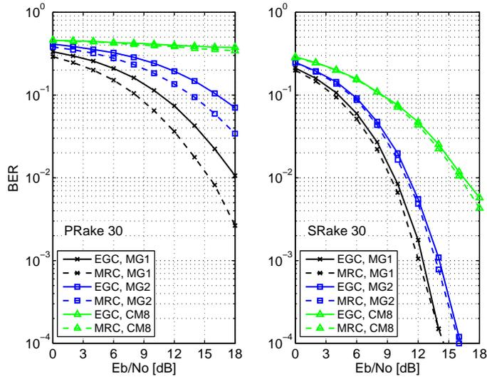
Figure 5.4: Comparison of EGC and MRC combining using 30 fingers of PRake (left) and SRake (right) on MG1, MG2 and CM8.
