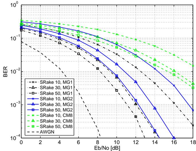
Figure 5.3: Comparison of BER of different number of fingers of SRake with MRC combining on MG1, MG2 and CM8.
