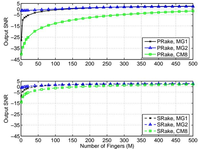
Figure 5.1: Output SNR vs Number of RAKE fingers on MG1, MG2 and CM8 PRake (top) and SRake(bottom).
