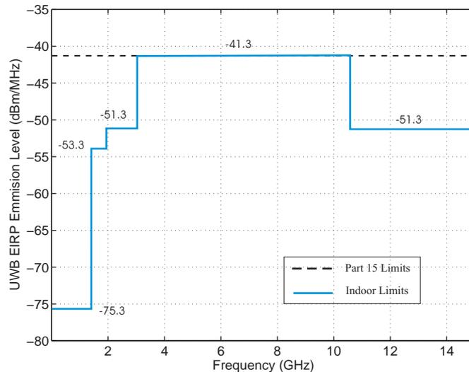
Figure 1.1: FCC allocated spectral mask for indoor ultra wideband communication systems [3].
