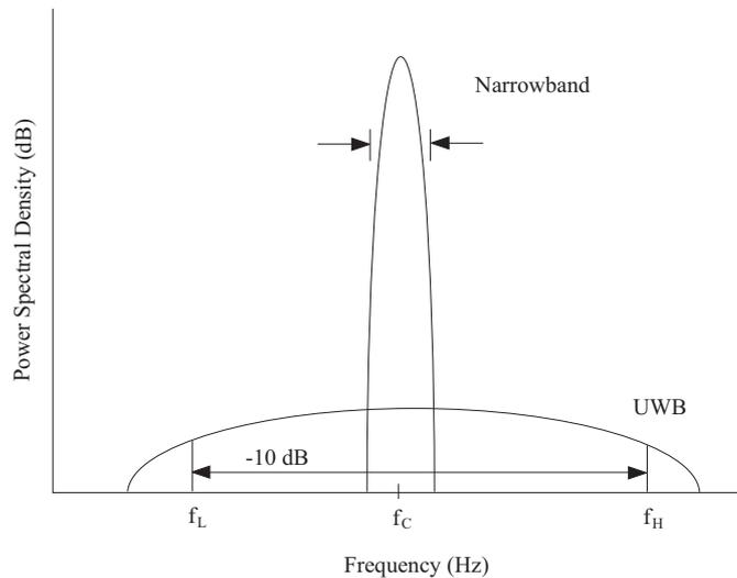
Figure 1.2: Comparison of the Fractional bandwidth of a narrowband and ultra wideband communication system [6].
