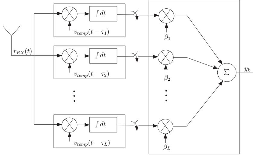
Figure 4.1: A RAKE receiver structure for TH-IR UWB system.
