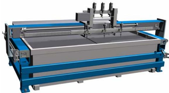
Figure 1. Example of a water jet cutting machine.
