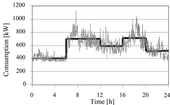
**Figure 5. The amount of hot tap water produced by the reference control scheme (indicated by the thick line, 0% surplus production), compared to the 5-day average consumption.**
