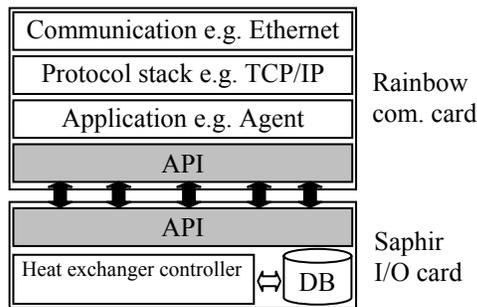
**Figure 3. The Rainbow communication and computation card is here shown on top of the Saphir hardware interface card.**
