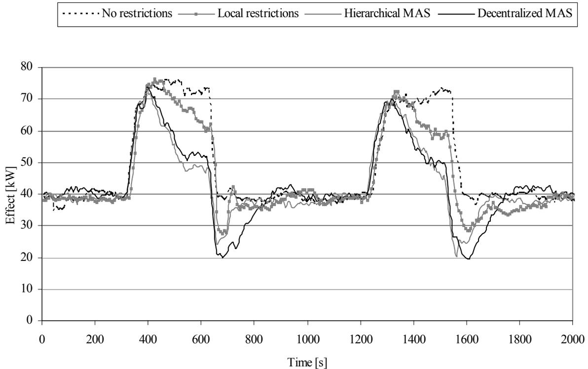
**Figure 8. Total system energy consumption for the four control strategies. The desired global consumption is 50 kW.**
