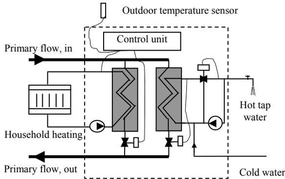
**Figure 2. A substation consisting of heat exchangers (the shaded boxes), control valves, pumps and a control unit. The household heating system (radiators) is controlled by the control unit, using information about actual outdoor temperature.**
