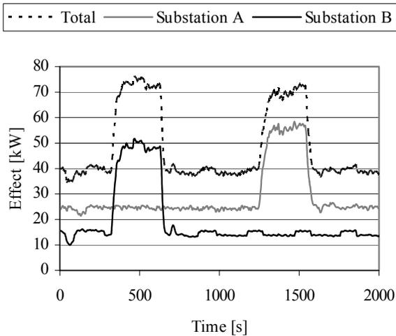
**Figure 7. Household heating and hot water tapping from two substations.**
