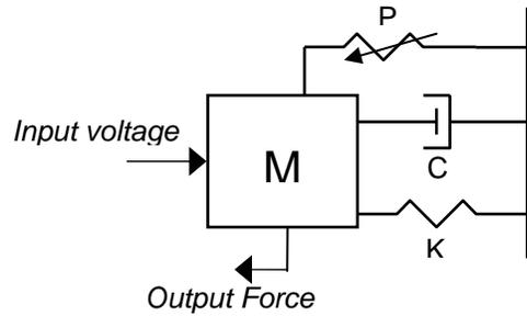
Figure 5.1. Simulation model used to test the algorithm. The values used are  $m = 0.024 \text{ kg}$  ,  $C = 1.5 \text{ Ns/m}$  ,  $K = 1.6 \cdot 10^6 \text{ N/m}$  and  $P = 1.6 \cdot 10^8 \cdot x^3 \text{ N/m}$
