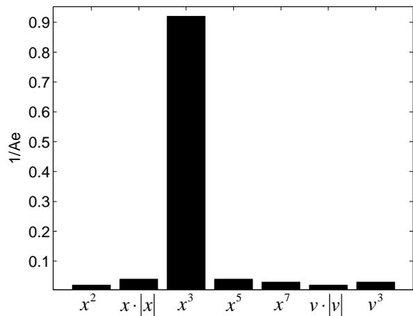
**Figure 3.5:** The presence of a cubic stiffness could clearly be seen. Nonlinear functions that depend on the velocity, as well as the unphysical  $x^2$ , were included for comparison.
