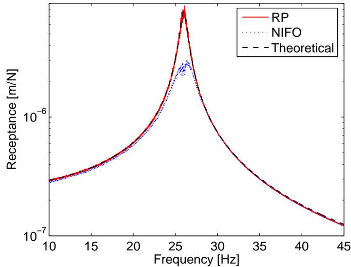
**Figure 4.2: Estimated linear system - comparison between the two models shown in Figure 4.1. After averaging a large bias error is left with NIFO while the reverse-path formulation performs better since the *H1-estimator* minimizes the effect from noise at the output.**
