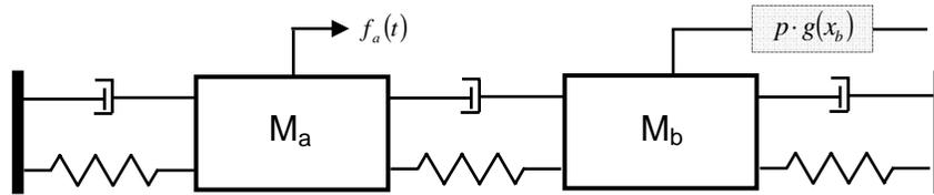
**Figure 2.2: A nonlinear system with two degrees of freedom and a nonlinear element connected to the second dof. The nonlinearity is described with a nonlinear operator  $g(\cdot)$  with a coefficient  $p$ .**
