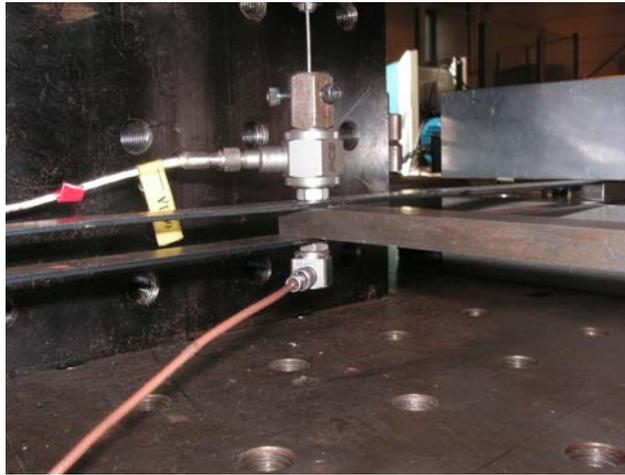
**Figure 5.4: A detail view of the experimental setup. A force transducer and an accelerometer are used at the selected measurement point.**
