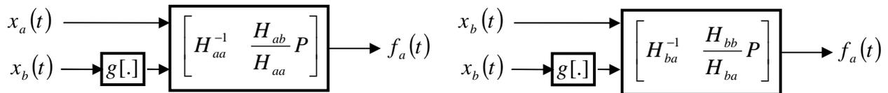
**Figure 2.3: Reverse-Path (RP): Two MISO analyses are performed and using the reciprocity of the underlying linear system  $H_{aa}^{-1}$ ,  $H_{ba}^{-1}$  and the nonlinear coefficient  $P$  can be identified. Here,  $g(\cdot)$  is a nonlinear operator.**
