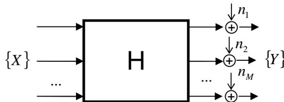
**Figure 2.1: A Multiple-Input-Multiple-Output Model (MIMO) with noise on the outputs.**
