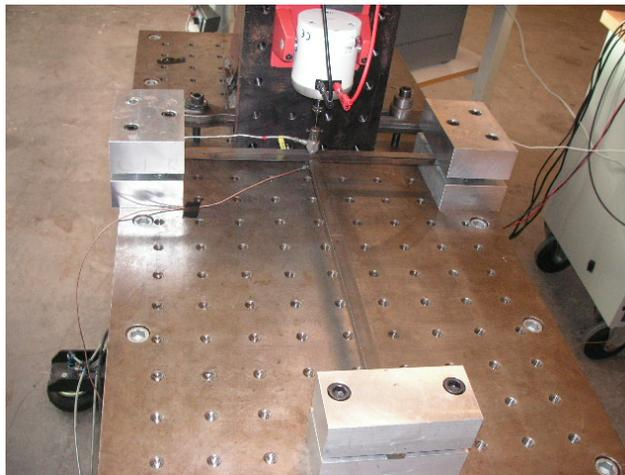
**Figure 5.3: The complete setup for the experimental test. The structure is fixed to a rigid table and a shaker is used to excite the structure.**
