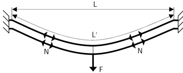
**Figure 5.2: The transversal beams will behave nonlinearly at higher displacements. As the force is increased the beams becomes longer than the original length  $L$ , and an axial force is introduced along the beams. The stiffness will therefore increase. This effect is known as geometric nonlinearity.**
