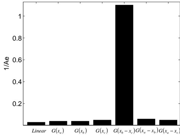
**Figure 3.4:** The method correctly detects that the nonlinear element is connected between  $x_b$  and  $x_c$ . The true nonlinearity in the black-box system was a cubic function that depends on the relative motion between  $x_b$  and  $x_c$ .
