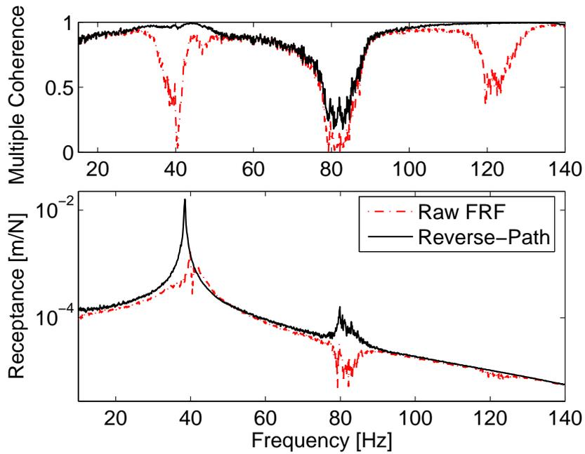
**Figure 5.5: The Raw FRF (linear theory) compared with the linear system estimated with reverse-path technique. A cubic function is used to describe the nonlinearity. As shown, the FRF and the coherence are improved at the resonance and at three times the resonance frequency.**
