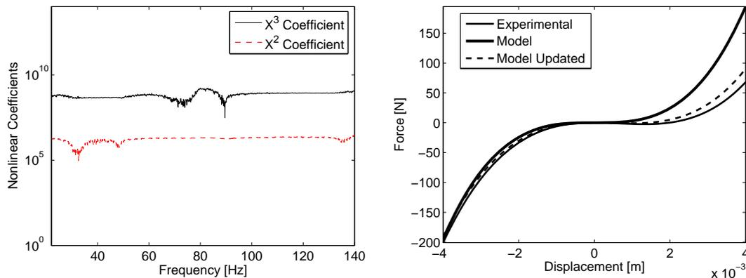
**Figure 5.8: The nonlinear coefficients (left) and the estimated nonlinearity compared with the model (right). The nonlinear static model could be updated with the experimental parameters.**
