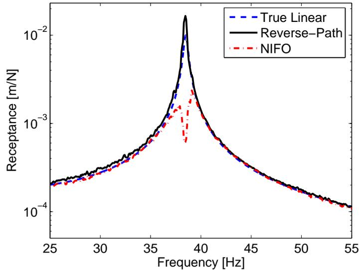
**Figure 5.7: The estimated linear system with different methods. The true linear FRF, used as reference, was measured at very low excitation. As shown, the estimated linear system with NIFO techniques gives larger amplitude errors.**
