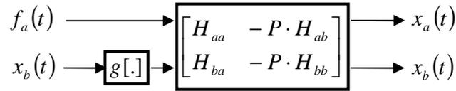
**Figure 2.4: Nonlinear Identification Through Feedback of Outputs (NIFO):** A single MIMO analysis is performed and using the reciprocity of the underlying linear system  $H_{aa}$ ,  $H_{ba}$  and the nonlinear coefficient  $P$  can be identified. As in Figure 2.3,  $g(\cdot)$  is a nonlinear operator.
