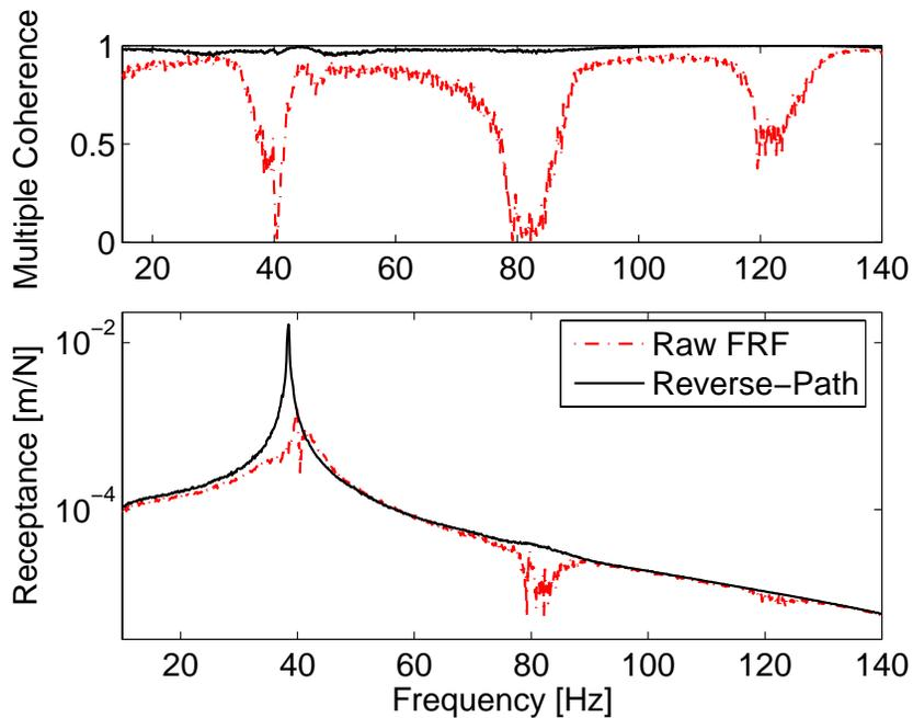
**Figure 5.6: The Raw FRF (linear theory) compared with the linear system estimated with reverse-path technique. A cubic- and a square- function are used to describe the nonlinearity. As shown, the FRF and the coherence are considerably improved over the frequency range.**
