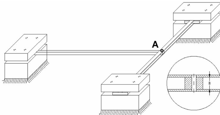
**Figure 5.1: The structure used in the experiment consists of a clamped beam with two fixed transversal beams connected at point B. The clamped beam has a cross section of (15x8) mm with a free length of 420 mm and the two transversal beams has a cross section of (13x1.4) mm and free length 242 mm.**
