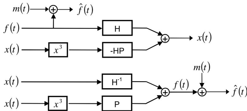
**Figure 4.1: Analysis of a duffing system with a NIFO model (above) and the reverse-path technique (below). A small amount of noise is added to the force channel as shown in the figure.**
