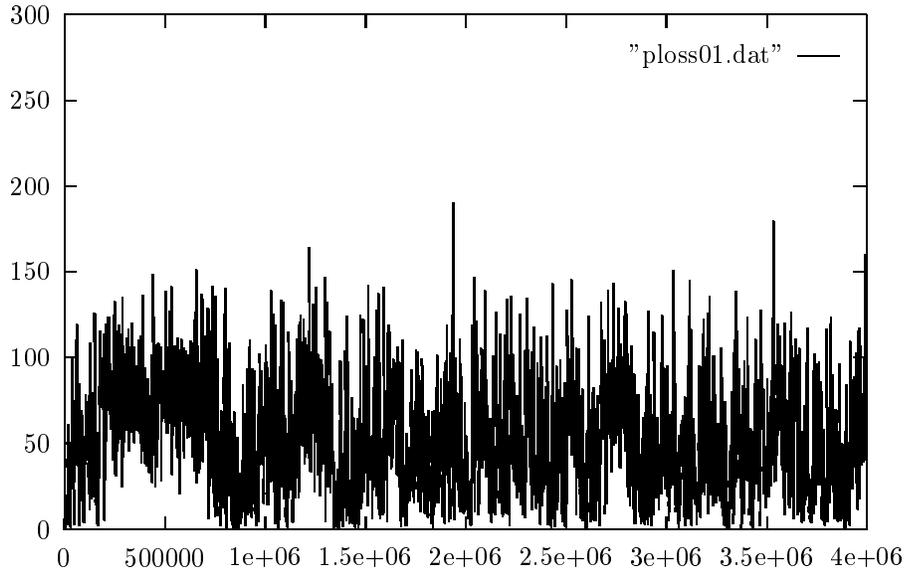
Figure 3: The aggregate server to client traffic over a lossy link (1% %losses) in a simulation with approx. 300 clients and servers. The traffic shown is at the link layer and is being “shaped” by TCP flow control. The vertical axis shows the number of Kbytes aggregated over 1 second intervals (horizontal axis)
