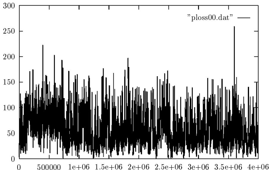
Figure 2: The aggregate server to client traffic over a lossless link in a simulation with approx. 300 clients and servers. The traffic shown is at the link layer and is being “shaped” by TCP flow control. The vertical axis shows the number of Kbytes aggregated over 1 second intervals (horizontal axis)
