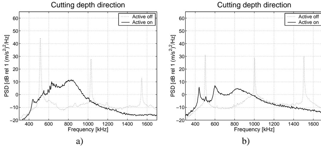
Figure 5: Power spectral densities of boring bar vibration in the cutting depth direction with and without active vibration control using in a) a  $0^\circ$  and in b) a  $30^\circ$  active boring bar. The cutting speed was 80 m/min, the cutting depth was 1.0 mm and in a) the feed rate was 0.2 mm/rev and in b) 0.3 mm/rev.
