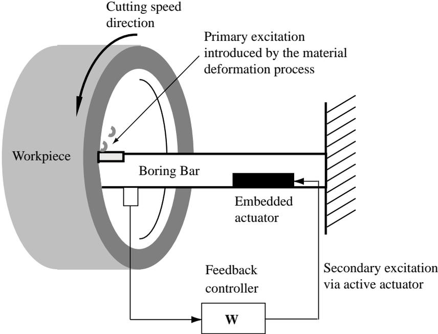
Figure 1: A schematic figure of active vibration control in a boring operation.
