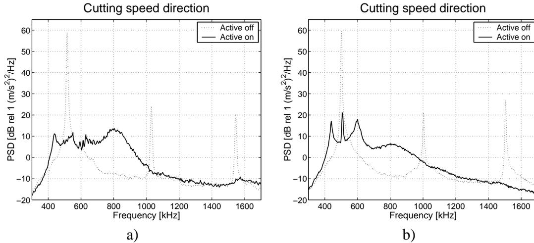
Figure 4: Power spectral densities of boring bar vibration in the cutting speed direction with and without active vibration control using in a) a  $0^\circ$  and in b) a  $30^\circ$  active boring bar. The cutting speed was 80 m/min, the cutting depth was 1.0 mm and in a) the feed rate was 0.2 mm/rev and in b) 0.3 mm/rev.
