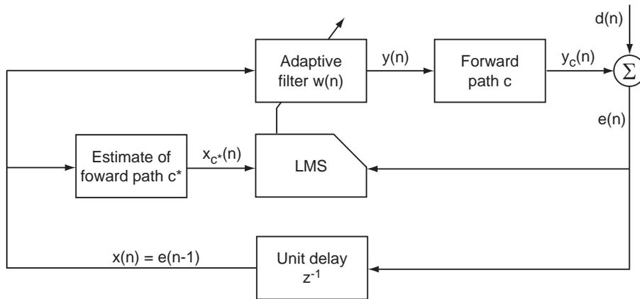
Figure 2: Block diagram of the feedback filtered-x LMS algorithm.
