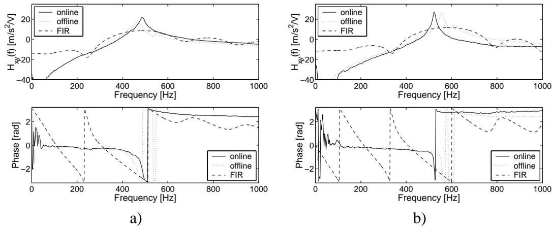
Figure 3: Frequency response function estimates of the forward path during continuous cutting operation, online, and when the boring bar is not in contact with the workpiece, offline. Fourier transformed offline FIR filter estimate of the forward path. In a)  $0^\circ$  and b)  $30^\circ$  active boring bar.
