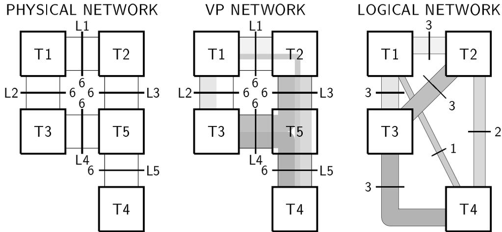
Figure 1: *Formation of a logical network of virtual paths.*
