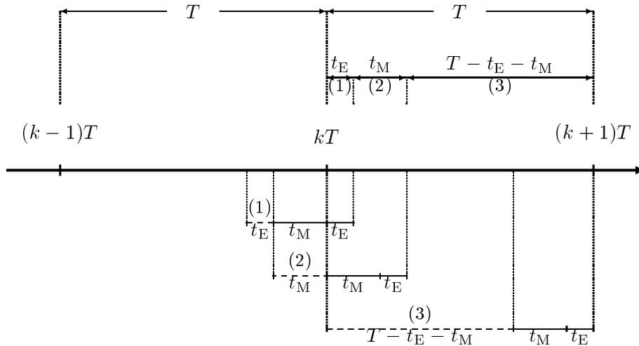
Figure 3: Model for estimating a variable traffic.
