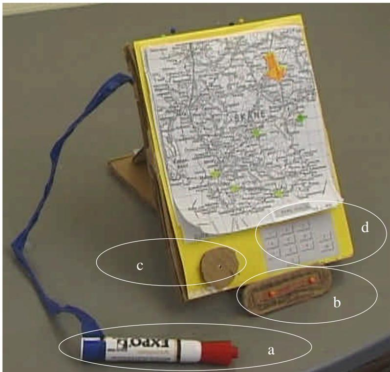
*Picture 5 The mockup of the NaviMap. The white board pen is representing a hand-held barcode reader. The NaviMap is on the picture placed in a docking station.*
