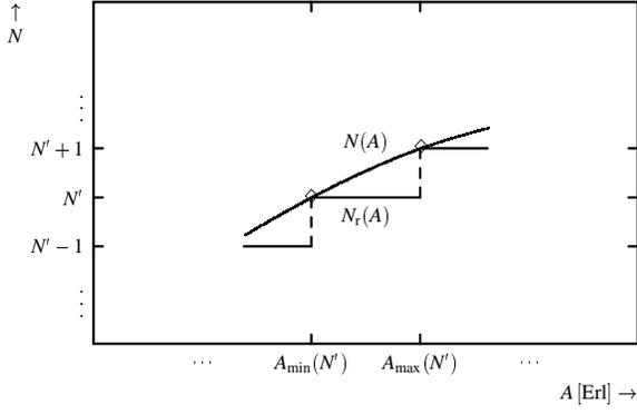
Figure 1: Required number of connections  $N_r(A)$ , critical points ( $\diamond$ ) and an optimal approximation function  $N(A)$ .
