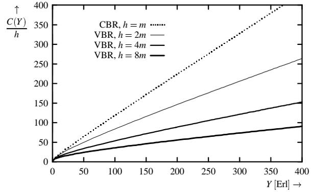
Figure 2: Approximated required capacity above load for CBR and VBR on/off connections,  $P_{\text{block}} = 10^{-2}$ ,  $P_{\text{loss}} = 10^{-9}$ , buffer size  $K = hb$ .
