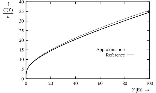
Figure 3: Approximated and reference values of required capacities above load for VBR on/off connections,  $h = 8m$ ,  $P_{\text{block}} = 10^{-2}$ ,  $P_{\text{loss}} = 10^{-9}$ , buffer size  $K = hb$ .
