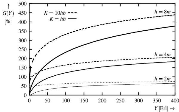
Figure 5: Gain above load for VBR on-/off connections,  $P_{\text{block}} = 10^{-2}$ ,  $P_{\text{loss}} = 10^{-9}$ .
