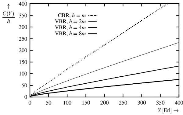
Figure 4: Approximated required capacity above load for CBR and VBR on-/off connections,  $P_{\text{block}} = 10^{-2}$ ,  $P_{\text{loss}} = 10^{-9}$ , buffer size  $K = 10hb$ .
