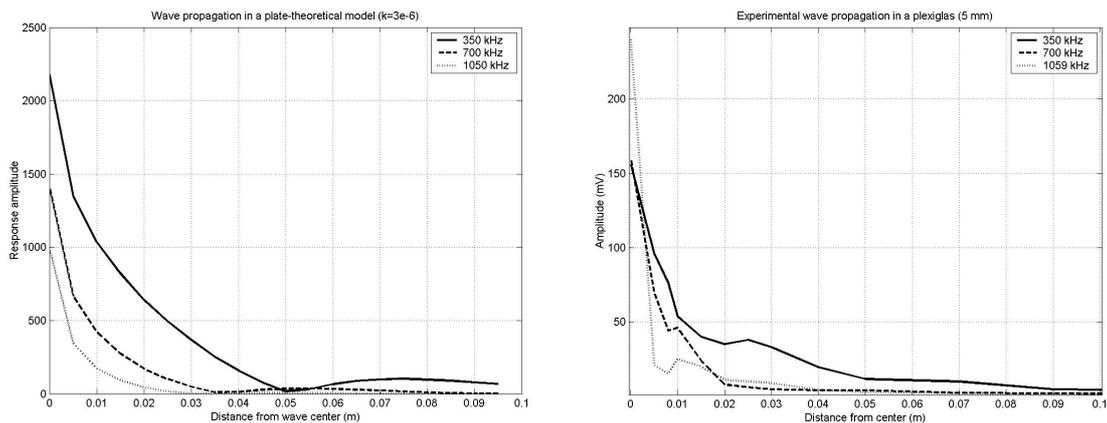
Figure 7. Wave propagation of three standing waves - simulation (left) and experiment (right).
