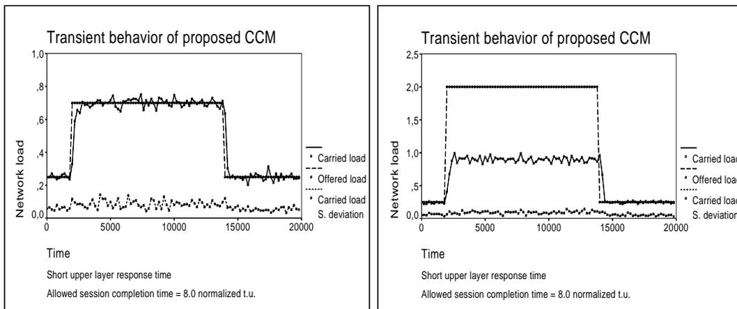
Fig. 7. The transient behavior of the proposed CCM at the single step loads of 0.7 and 2.0 respectively. The dashed line represents the offered network load and the solid line represents the carried load while utilizing the proposed CCM. Time is not equivalent to time units (t.u.).
