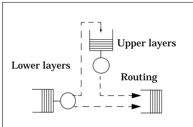
Figure 5. Queueing model of node interior.
