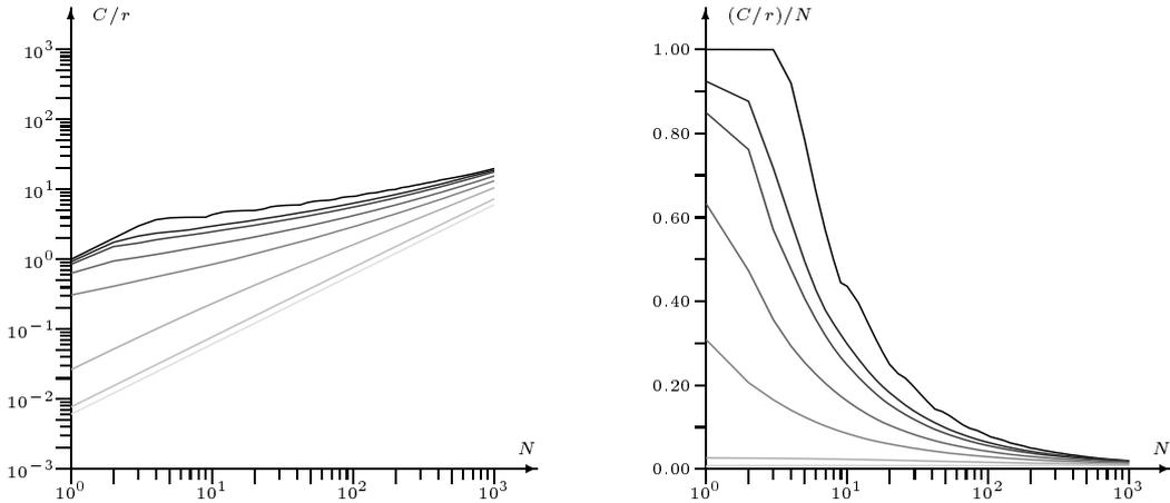
Figure 1: *Capacity requirements (left) and average bandwidths (right) assigned per call for  $K = 0, 1, 2, 5, 10, 20, 50, 100$ ,  $p_a = 0.5\%$  and  $\epsilon = 10^{-8}$ .*
