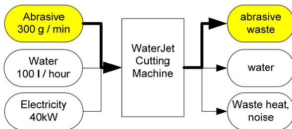
Figure 2. Expanding the view of the Waterjet Cutting Machine to include other required energy and material flows in the cutting process. The abrasive is highlighted due to having the greater environmental impacts.
