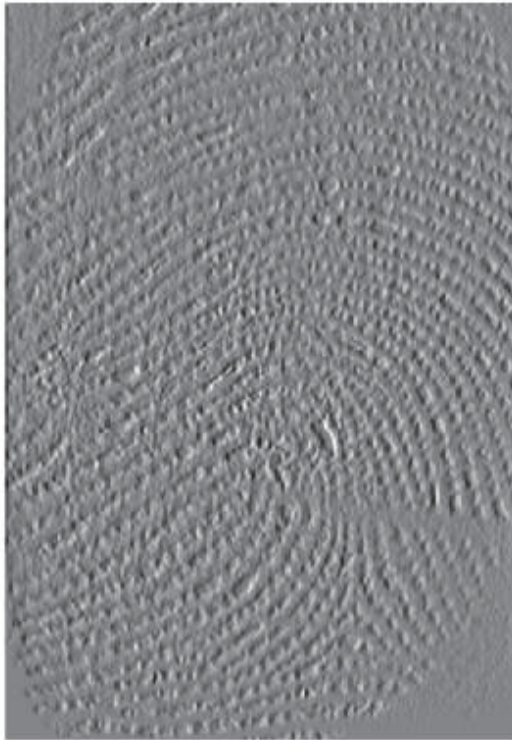
Figure 3.6 Gradient of the Image in x-direction
