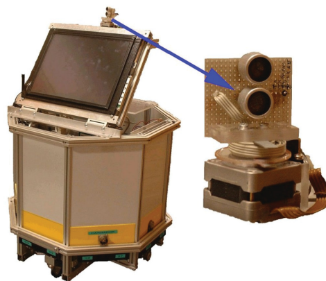
Figure 2.5: Piezoceramic Transducer Vertically Aligned And Mounted Onto A Stepper Motor [19]
