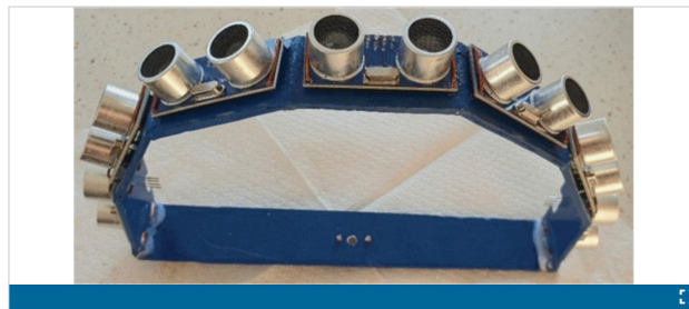
Figure 2.3: Ultrasonic System For Cartography [24]
