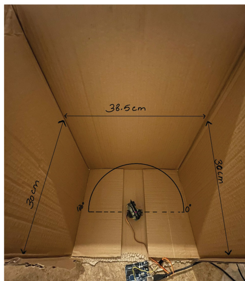
Figure 5.10: Prototype Scanning The Three Walls Of The Box
